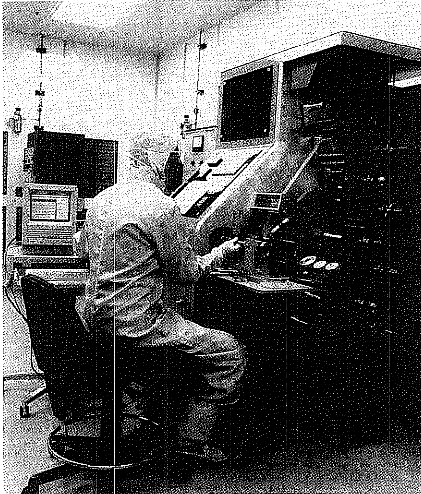
Fig. 8 Fabricating a Capacitor on the CL805 Winding Machine
