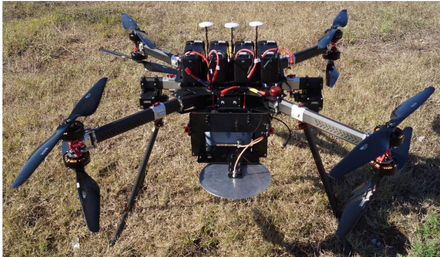
Figure 2.2.1 - GD-40X UAS with mounted measurement equipment
