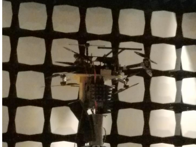
Figure 5.1 - UAS in anechoic chamber
