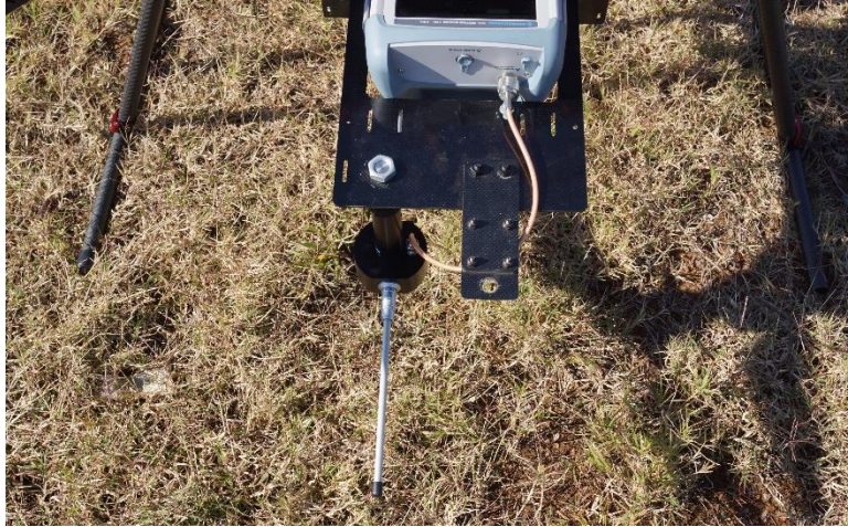
Figure 2.2.4 - Glideslope dipole antenna on UAS
