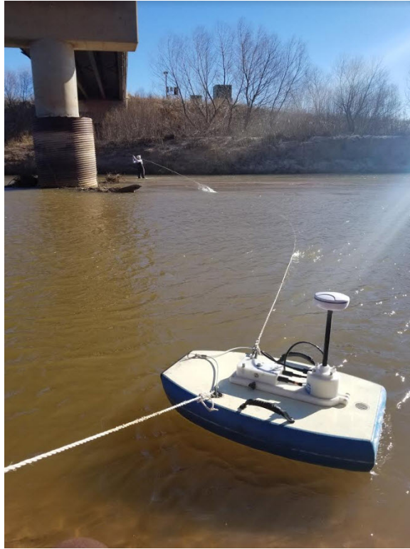
Figure IV.9: Acoustic Doppler Current Profiler
