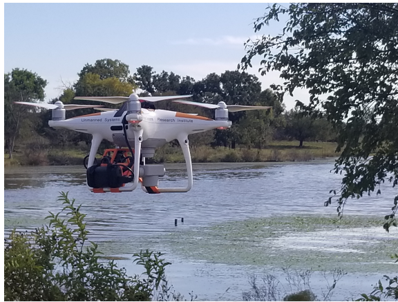
Figure I.1: Phantom 4 Pro with multiple photogrammetric sensors
