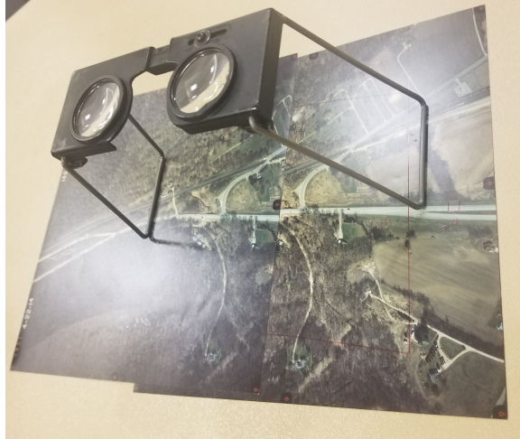
Figure I.2: stereoscope and matching pair of stereo images
