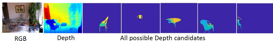
Figure 3.9: Example of segmented objects from three NYUD2 depth images. A candidate input depth image contains one of the ten objects (bathtub, bed, chair, desk, dresser, monitor, nightstand, sofa, table and toilet). The depth image has five possible candidate depth images.
