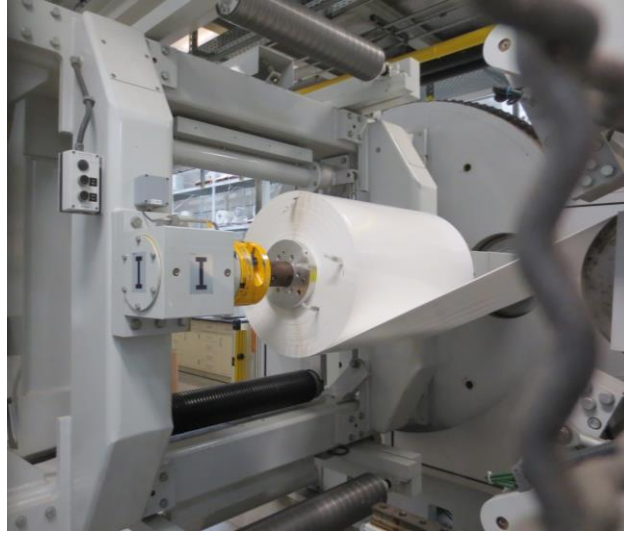
Fig. 4.9 Machine Set Up for Laminate Web Winding Tests
