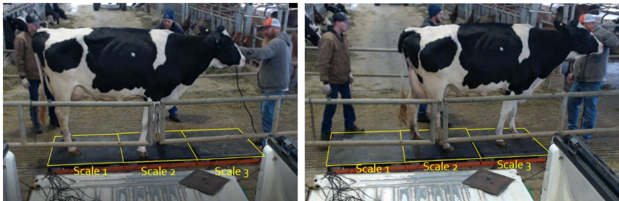
Figure 34 Dairy Cattle Static Weight collection. LEFT First ten seconds. RIGHT second ten seconds.
