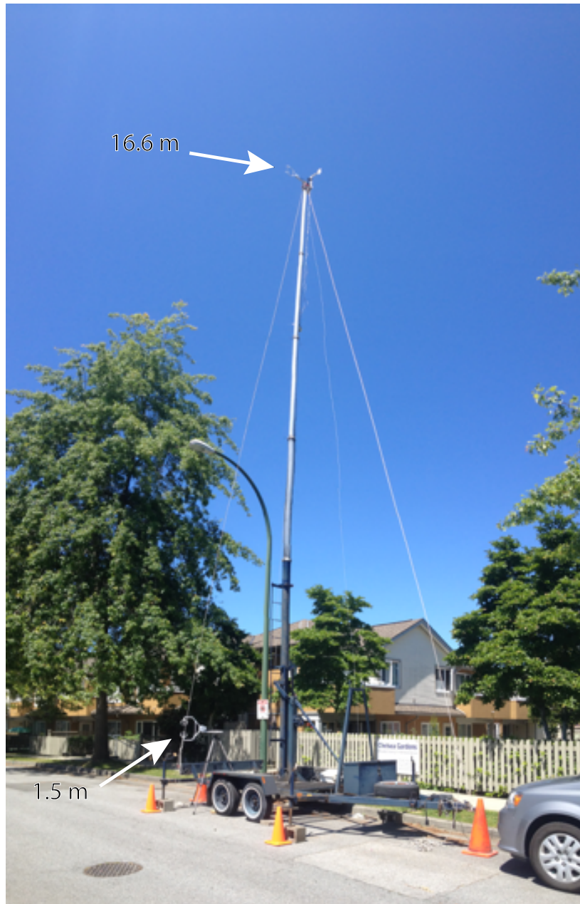
Figure 2.9: Mobile 3D sonic anemometer tower with both 3D sonic anemometer heights labelled
