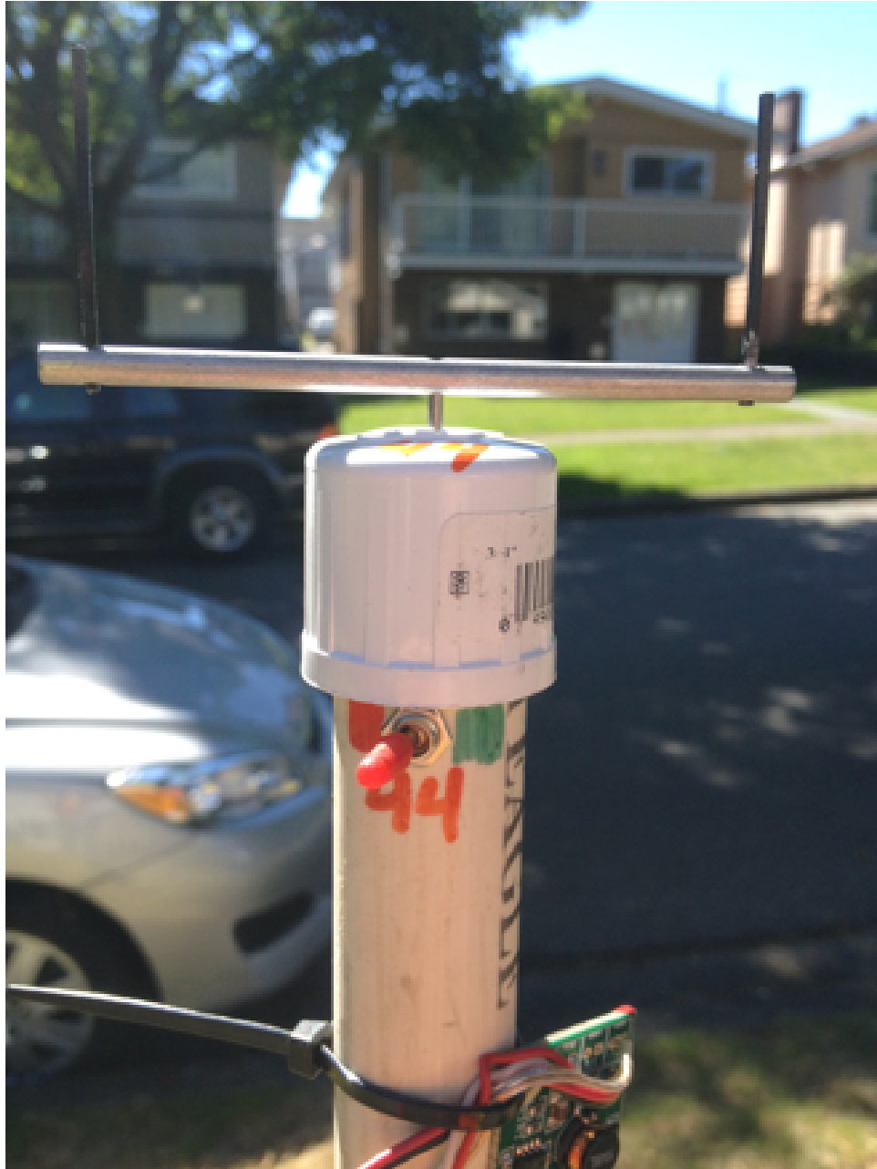
Figure 2.8: Close-up of one impact trap, based off of Thiessen et al. (2016)
