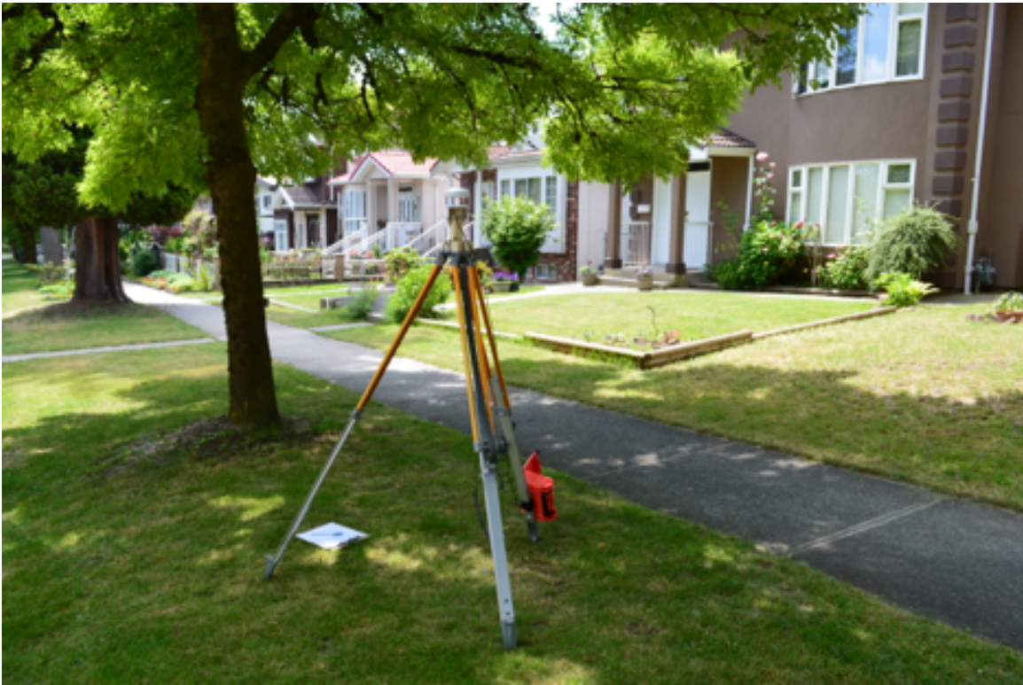
Figure 2.10: Example of a 2D sonic anemometer, based off of Gunawardena et al. (2018)
