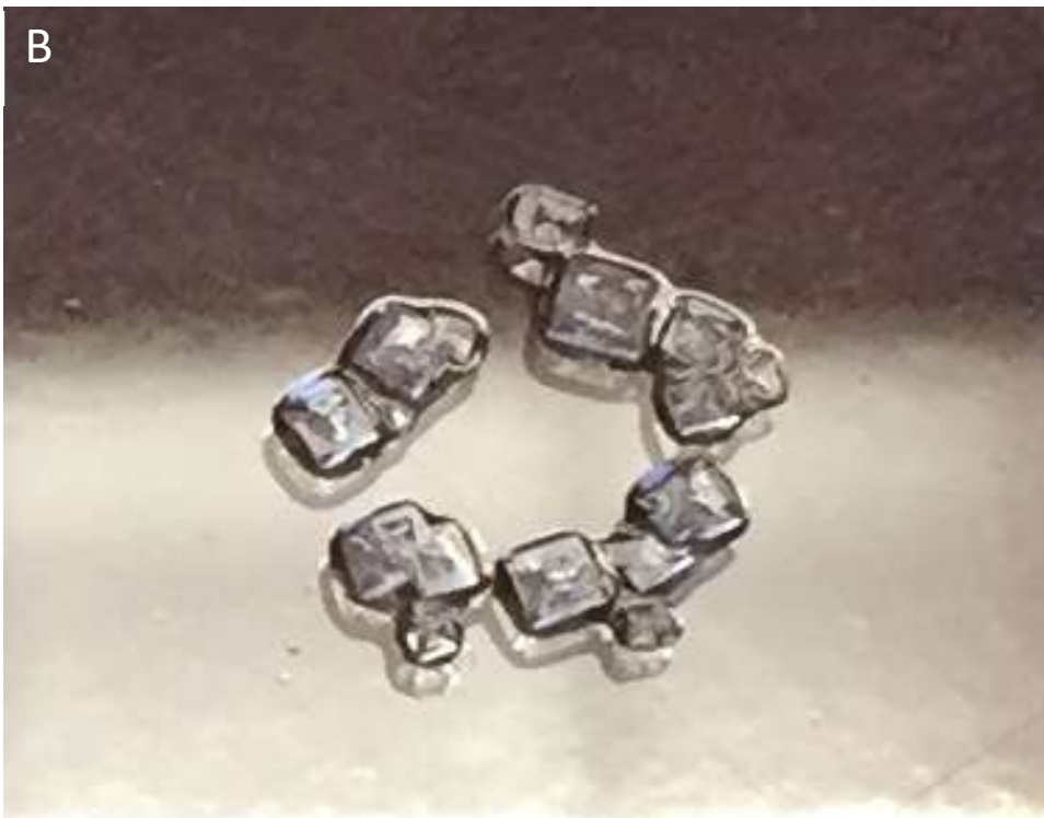
Figure 2.7. Precipitation of sucrose (A) and sodium chloride (B) from high concentration solutions on glass microscope slides.
