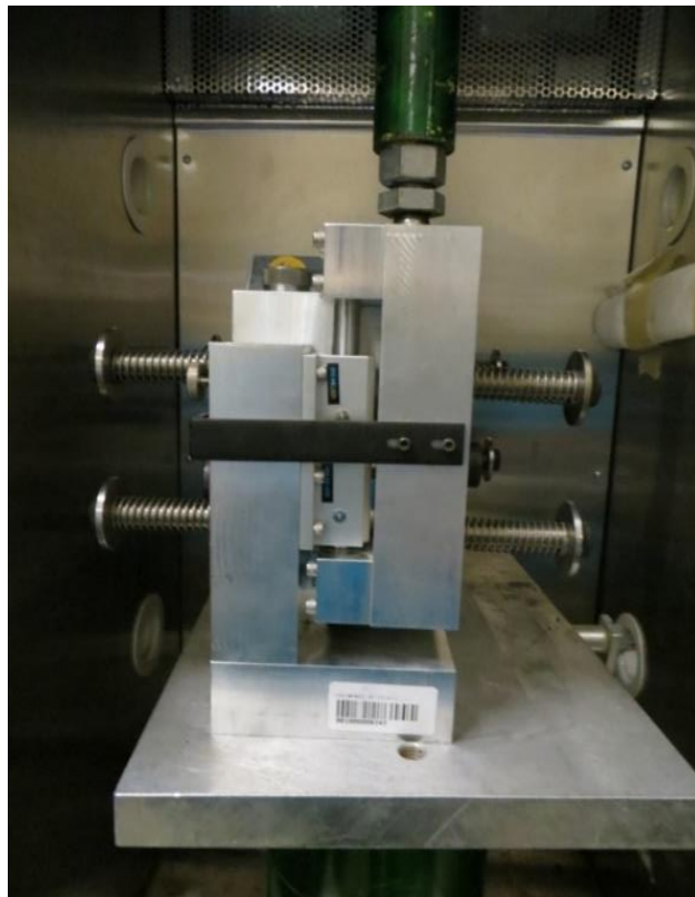
Figure 3.7 Louisiana Interlayer Shear Strength Test (LISST) Setup
