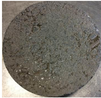
Figure 3.16 Asphalt Mix Sample after Polishing
