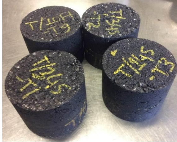
Figure 3.22 Compacted Samples for LISST Testing
