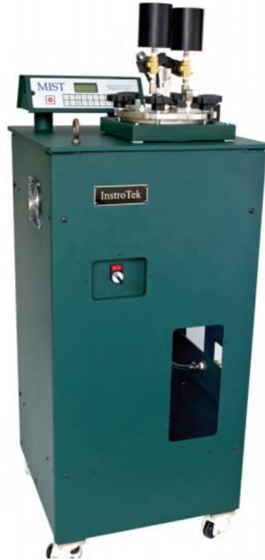
Figure 3.23 A Photographic View of MIST Device used for Moisture-Conditioning of Samples
