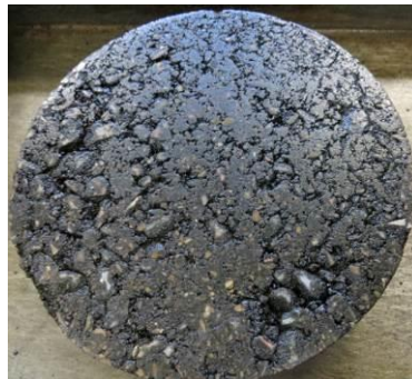
Figure 3.17 Asphalt Sample Surface after 120 hours of Oven Aging and Polishing
