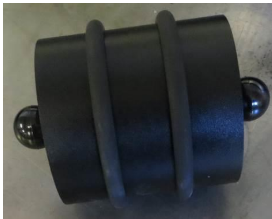
Figure 3.24 Steel Cylinder and Rubber O-rings Used for RTT Test
