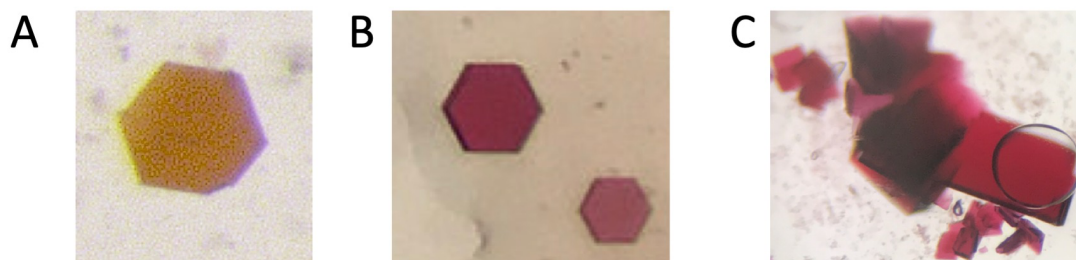
Figure 2.13. Shapes and colors of the crystals obtained in this study. A) Brown, ferric swMb III -H 2 O hexagonal shaped crystals indexed with the P6 space group. B) Violet-pink, ferrous swMb II -RNO (-PrNO, - i PrNO) hexagonal shaped crystals indexed with the P6 space group. C) Violet-pink, ferrous swMb II -RNO (-MeNO, -EtNO) thin plate crystals indexed with the P12 1 1 space group.
