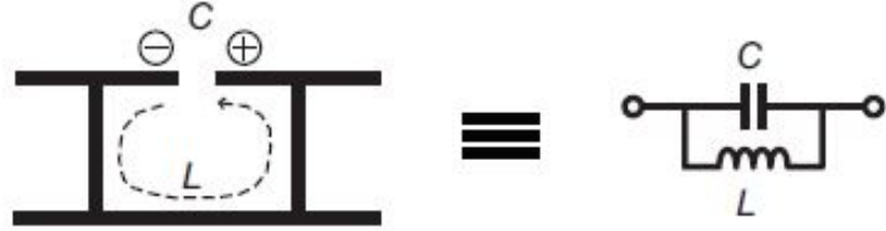
Figure 5.2: Lumped LC model for EBG analysis [2].
