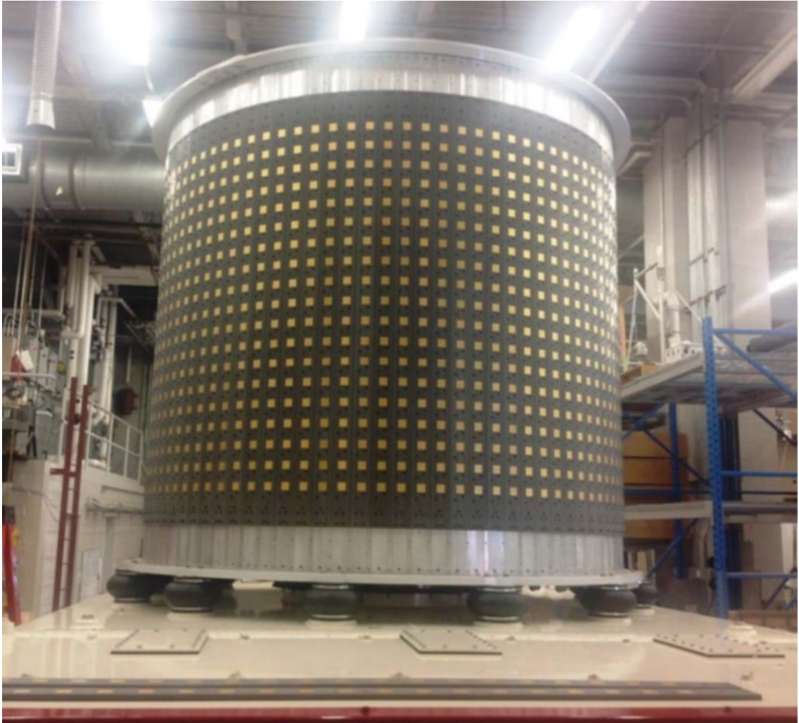
Figure 6.1: Cylindrical polarimetric phased array radar demonstrator.
