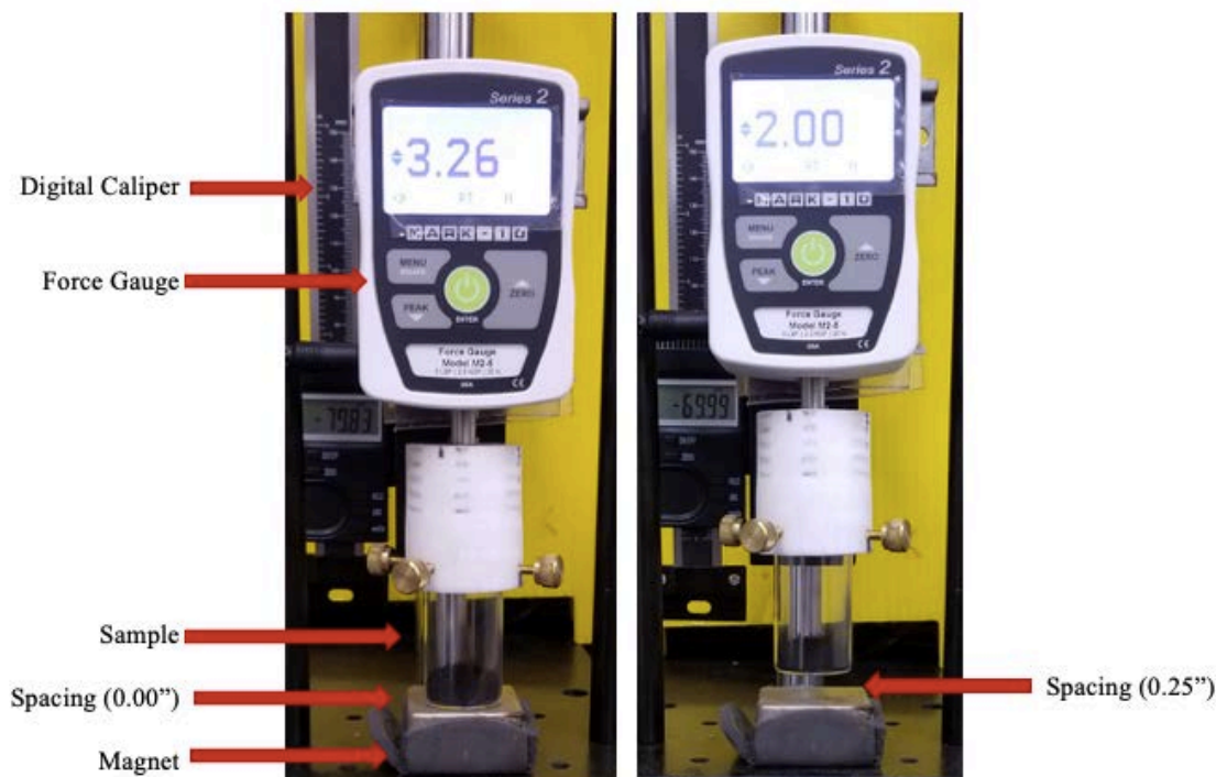
Figure 3.8 Instrument set-up for magnetic force measurement – 0.00” sample spacing (left); 0.25” sample spacing (right)
