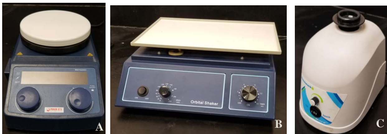
Figure 3.4 Mixing/Agitation Instruments; (a) magnetic heat/stir plate, (b) shaker plate, and (c) lab vortex
