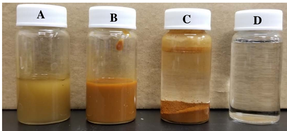
Figure 3.9 Commercial maghemite treatment test visualization, a) 1,000 ppm emulsion, b) 5 mg/mL MNPs, c) separated water and oil+MNPs, d) Treated water
