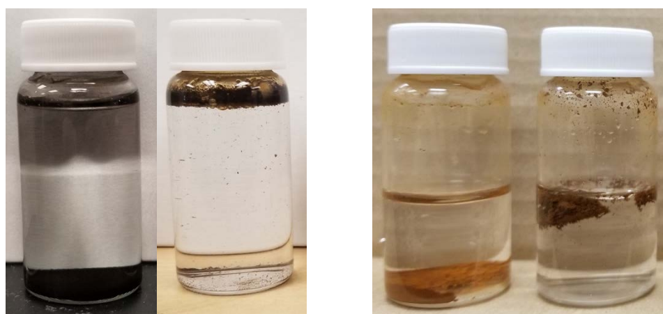
Figure 4.9 WCTC B005Jh maghemite gravity dominated vs. buoyancy dominated MNP conc. (left), commercial maghemite gravity dominated vs. buoyancy dominated (right) MNP conc.
