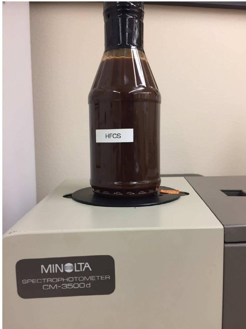
Fig. (2). BBQ sauce color measurement with a colorimeter.
