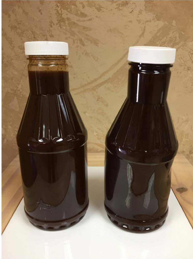
Fig. (1). Ordinary plastic bottle of BBQ sauce (left) and paneled (deformed) plastic bottle of BBQ sauce (right).
