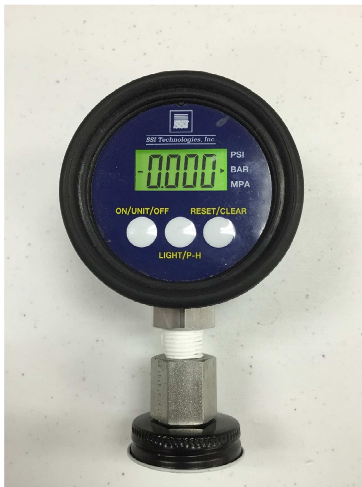
Fig. (4). Pressure gauge integrated with container cap to measure headspace pressure of a bottle.
