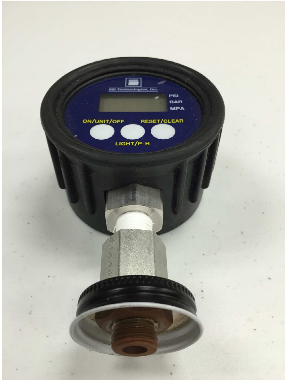
Fig. (5). Detail of pressure gauge sensor attachment to a screw-on container cap.
