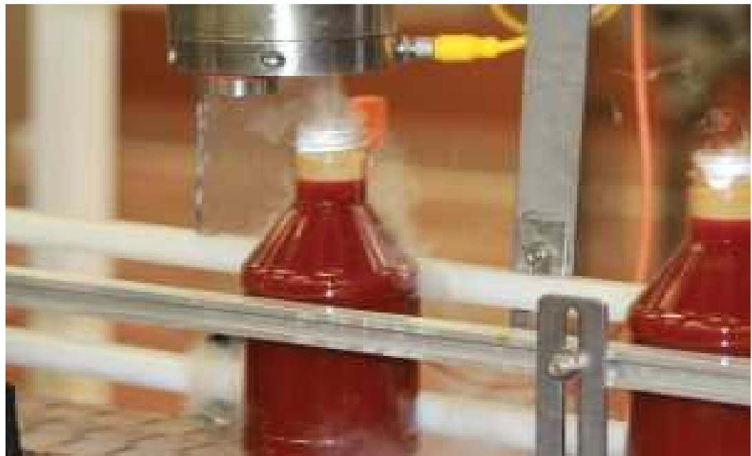
Fig. (3). Nitrogen gas dosed into a container of BBQ sauce just after hot filling.
