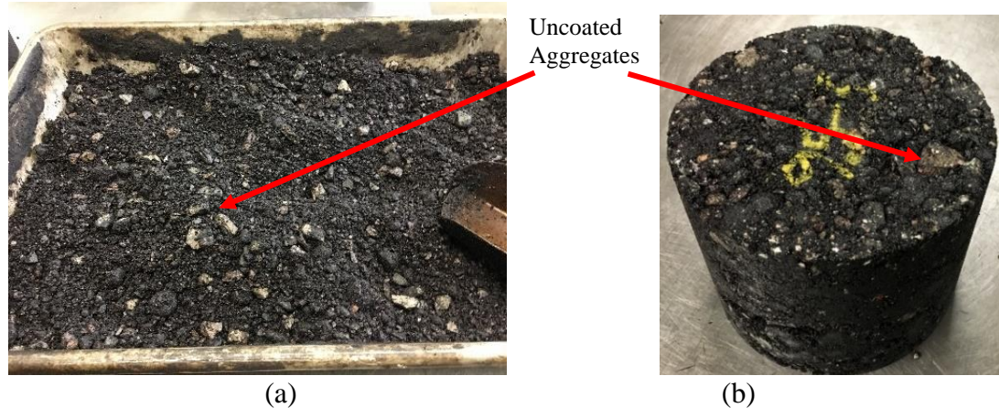
Figure 4.3 Uncoated Volumetric Samples at Lower Mixing and Compaction Temperatures (a) After Mixing and (b) After Compaction
