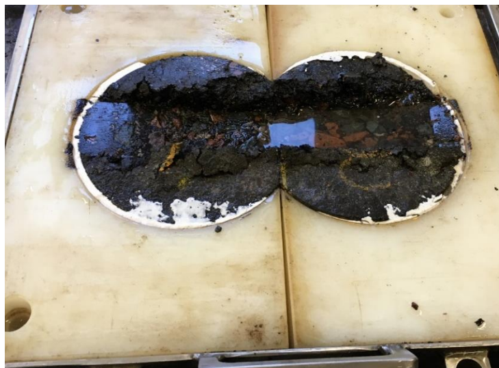
Figure 3.9 HWT Saw-Cut Molded Sample After Testing
