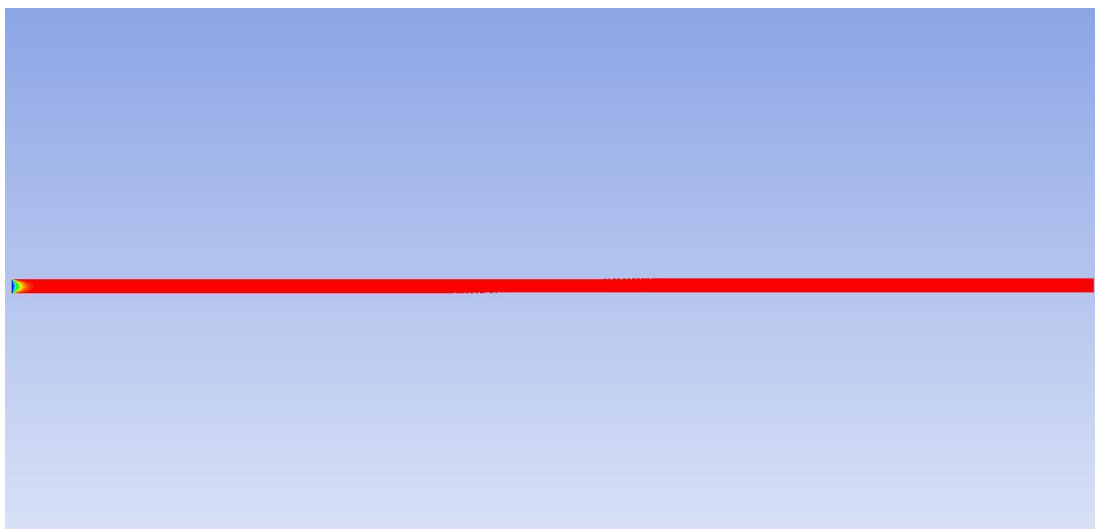
Figure 18. Temperature contour plot of the first 13 cm into the flow reactor before reaching the catalyst bed; blue represents room temperature and red shows the reactor at 300 °C
