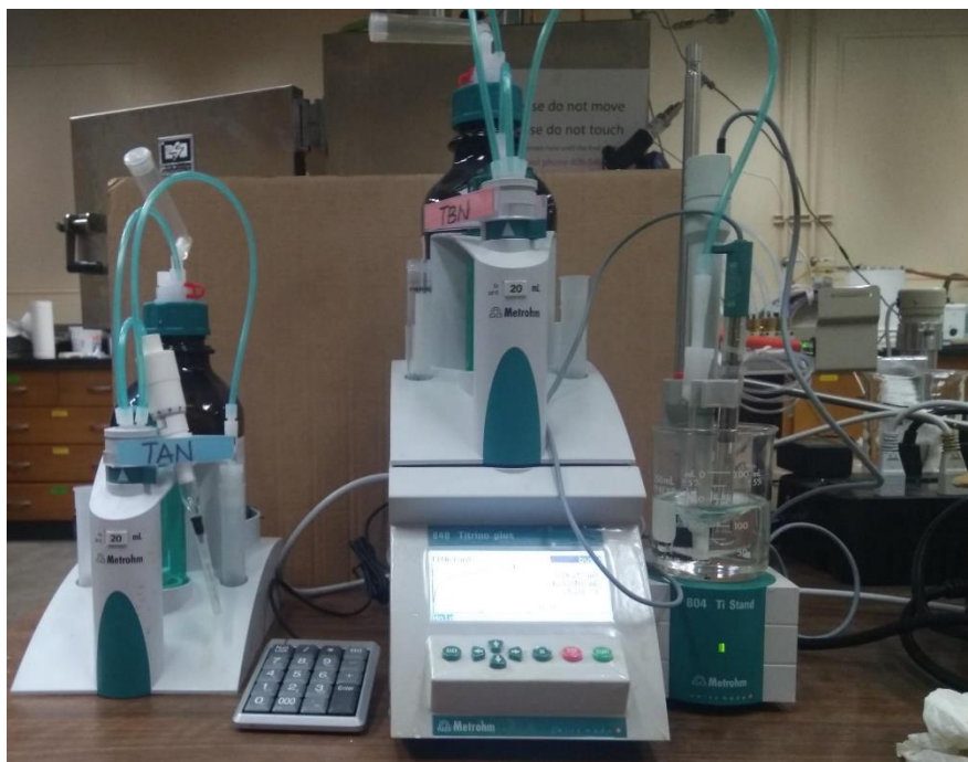
Fig. 19: Metrohm autotitrator (model 848) tritino plus with two exchangeable units, and a solvotrode electrode
