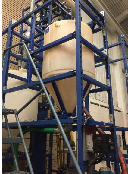
Figure 5. 3: Reservoir used to mix liquid phase with surfactant solution
