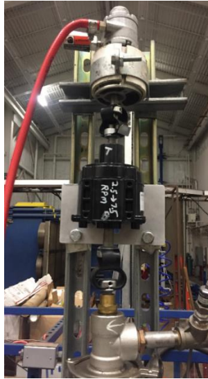
Figure 5. 13: Air motor used to rotate PTFE inner pipe of annulus
