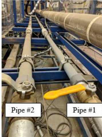
Figure 5. 6: Pipe viscometers used to characterize foam rheology
