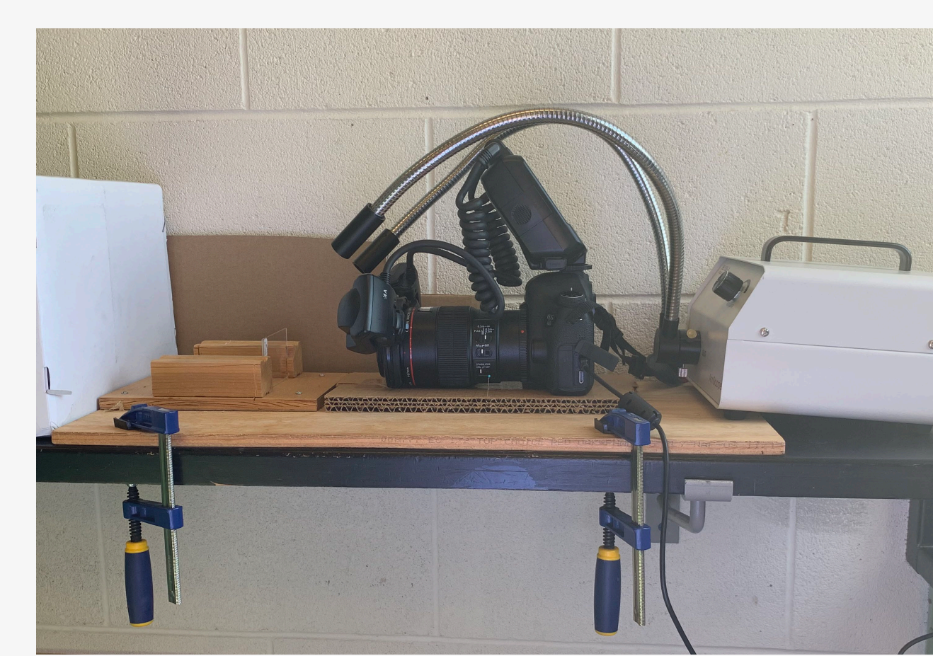
Figure 3: Canon EOS 6D with a 100mm Canon EF Macro lens and a Canon Macro Twin Lite MT-24 EX flash system.
