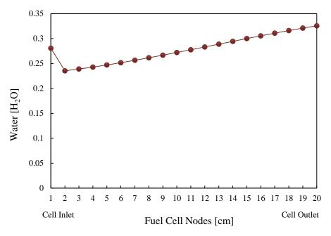
Figure 6.13. H<sub>2</sub>O profile across the fuel cells
