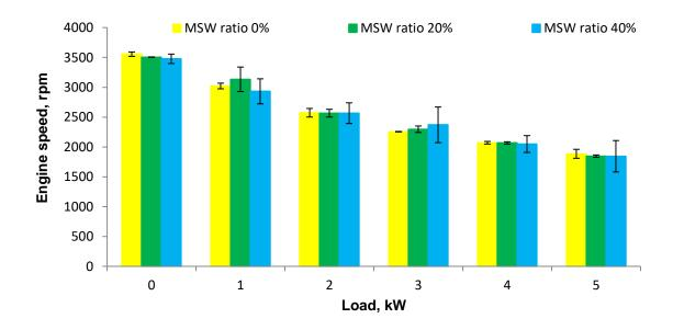
Figure 3.3. Speed of engine running on syngas generated at various MSW ratio (0, 20, and 40 wt.%)
