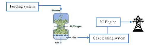
Figure 4.3. A schematic diagram of power generation derived from downdraft gasifier [51]
