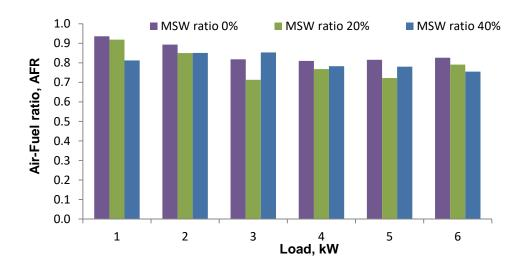
Figure 3.4. Air fuel ratio (AFR) of engine running on syngas generated at various MSW ratio (0, 20, and 40 wt.%)
