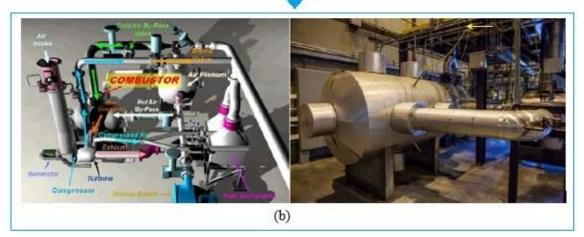
Figure 6.2. Schematic process of experiment: a) gasification plant at OSU, b) SOFC/GT hybrid power generation system at NETL
