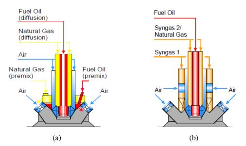
Figure 1.6. The modification of the GTs burner from: a) regular multi burner natural gas, to b) syngas type [104].
