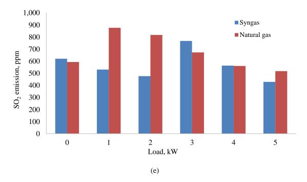
Figure 2.5. Emissions levels (ppm) of the engine operated on syngas and natural gas at varying load (kW): (a) CO<sub>2</sub>, (b) CO, (c) NO<sub>x</sub>, (d) HC, and (e) SO<sub>2</sub>
