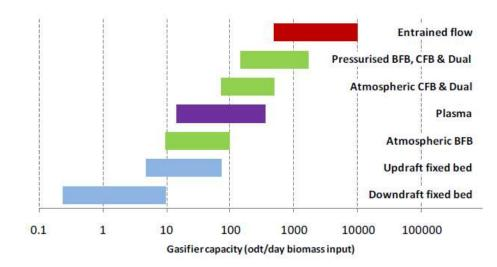
Figure 4.2. Gasifier technology versus capacity range [51]
