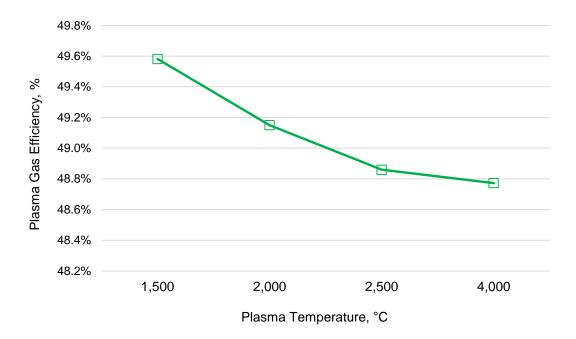
Figure 5.5. Effect of plasma temperature on plasma gasification efficiency (PGE)
