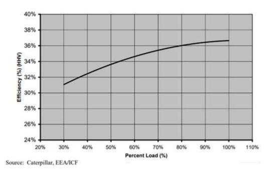
Figure 1.4. Efficiency of a natural gas ICE versus load [97]
