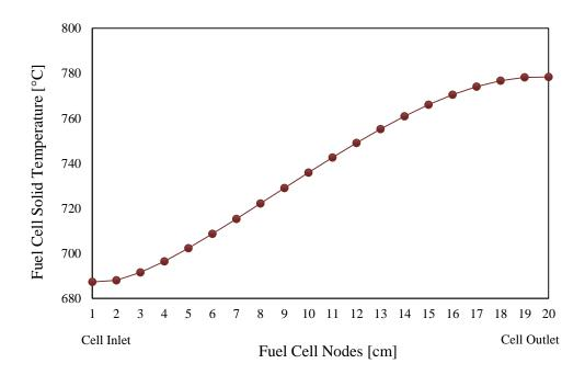
Figure 6.8. Fuel cell solid temperature across the fuel cells
