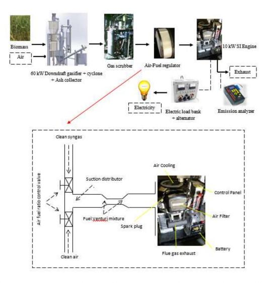
Figure 2.1. The process diagram of the power generation system with a modified air-fuel regulator coupled with a 60 kW of gasifier
