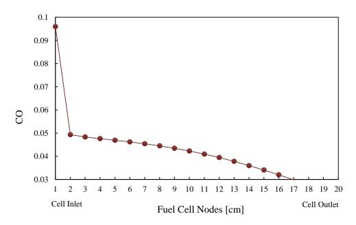
Figure 6.11. CO profile across the fuel cells
