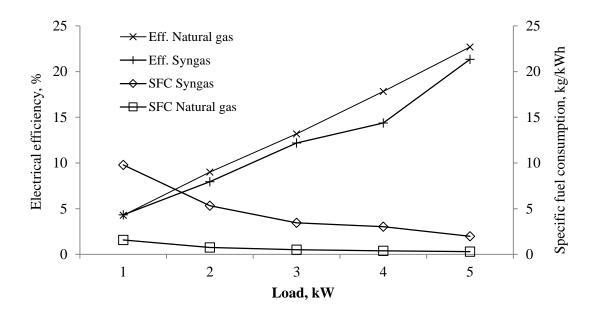
Figure 2.4. The electrical efficiency and specific fuel consumption of engine run syngas and natural gas
