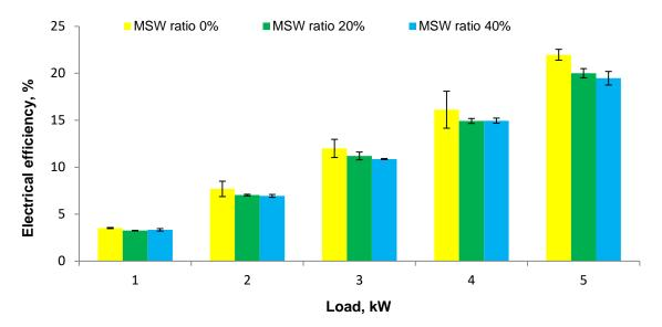
Figure 3.5. Electrical efficiencies of engine running on syngas generated at various MSW ratio (0, 20, and 40 wt.%)
