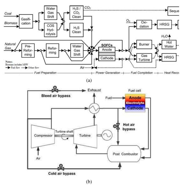
Figure 1.10. Schematics of a typical SOFC flow sheet using (a) various fuel types, and (b) a possible GT/SOFC integrated plant [24, 128]
