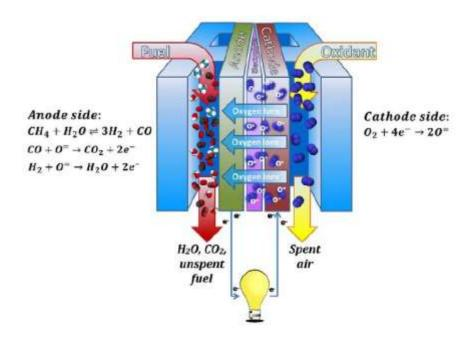
Figure 6.1. Basic diagram of an SOFC unit
