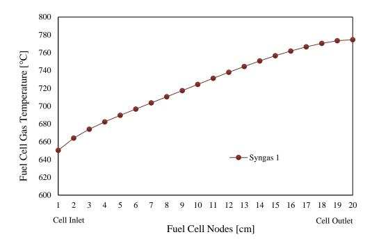
Figure 6.9. Fuel cell gas temperature across the fuel cells
