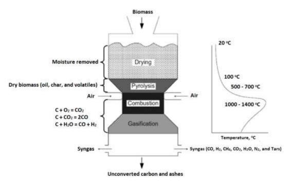
Figure 1.1. The steps of gasification and temperature profile [27]
