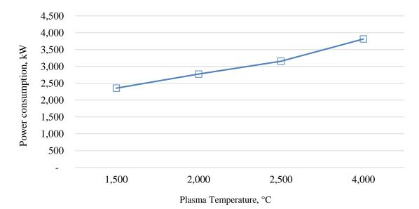
Figure 5.4. Effect of plasma temperature on energy consumption for generating plasma gas
