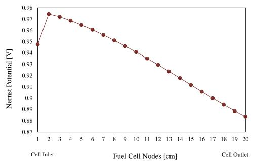
Figure 6.17. Nernst potential across the fuel cells
