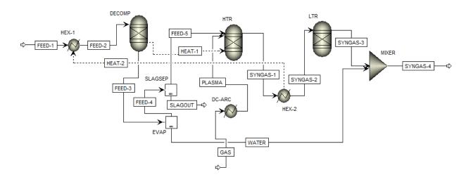
Figure 5.2. Process diagram of MSW plasma gasification
