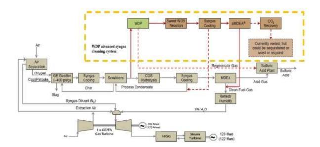
Figure 1.14. WDP advanced syngas cleaning system at Tampa Electric Company (TECO) [8]
