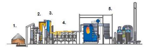
Figure 1.7. The Lahti Energia Plant, with the plant description: 1) fuel handling, 2) gasifier, 3) gas cooling, 4) gas filter, 5) gas boiler and flue gas cleaning [35]
