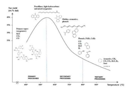
Figure 5.3. Tar yields in generic gasification process at different temperatures [220]
