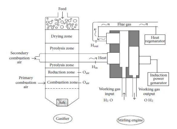
Figure 1.9. An updraft gasifier connected with a Stirling engine [112]
