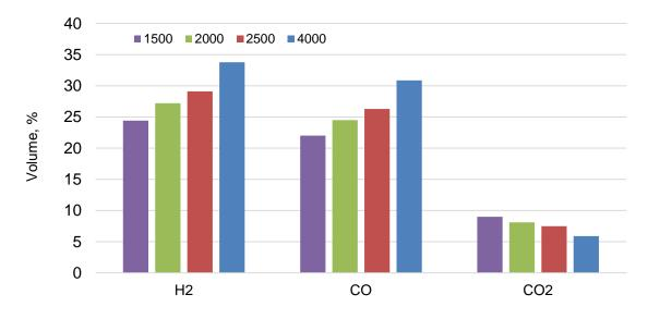
Figure 5.6. Syngas composition on different plasma temperatures
