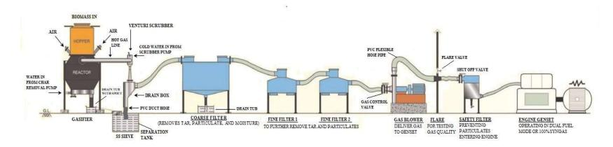
Figure 1.11. A schematic diagram of a 250 kW gasification based power generating system in Muzizi tea plant, Uganda [171]
