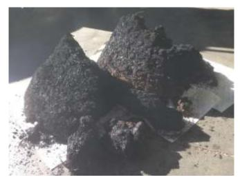
Figure 1.13. Samples of ash/slag collected from the ash collector from co-gasification of MSW and biomass, with a detailed performance of power generation reported by Indrawan et al. [60]
