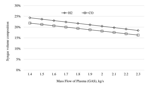
Figure 5.8. The effect of mass flow of plasma gas on syngas composition at 1,500°C
