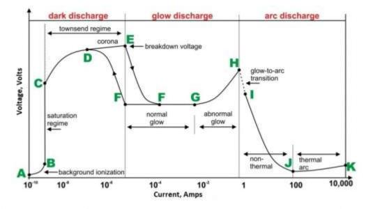
Figure 5.1. Types of plasma discharge based on voltage and current density [293]
