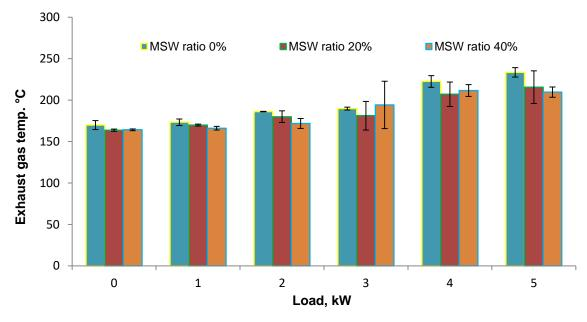
Figure 3.7. Exhaust gas temperature (EGT) with variable load
