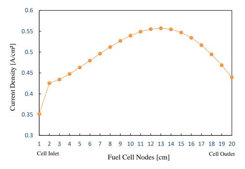
Figure 6.6. Current density profile across the fuel cells
