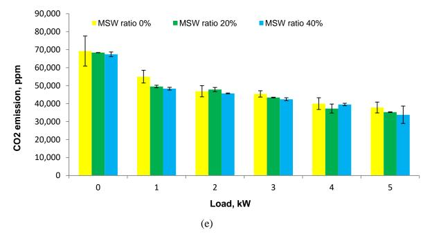
Figure 3.6. Emission profile (variation with change in load applied) of (a) CO, (b) NO<sub>x</sub>, (c) HC, (d) SO<sub>2</sub>, and (e) CO<sub>2</sub> of engine running on syngas generated at various MSW ratio (0, 20, and 40 wt.%)
