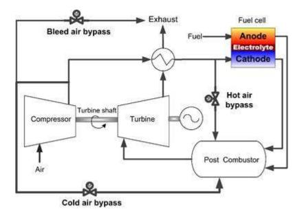
Figure 6.4. Simplified process diagram of SOFC/GT hybrid power generation system [312]
