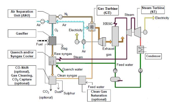
Figure 1.5. Sketch of an IGCC in principle [104].
