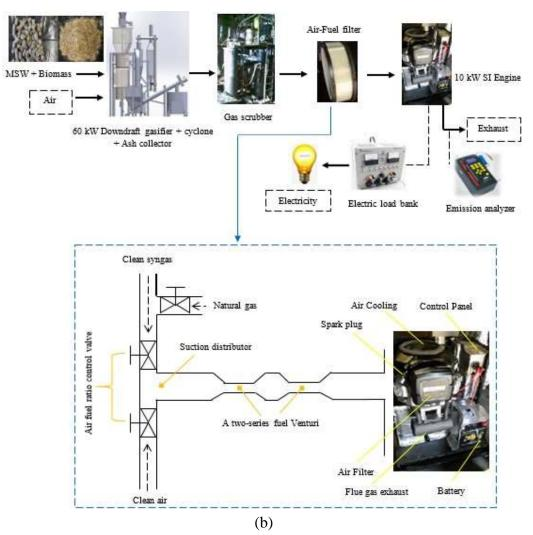
Figure 3.1. (a) Gasification system with total capacity of 60 kW and (b) detail experimental set-up with a modified air-fuel regulation
