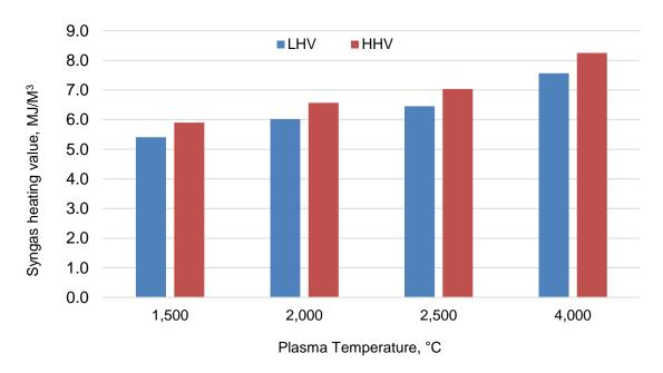
Figure 5.7. Effect of plasma temperature on syngas heating values
