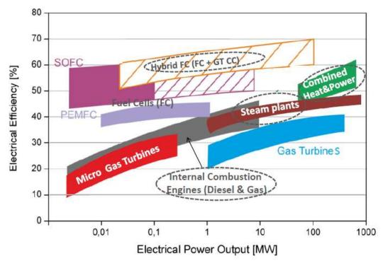
Figure 1.2. Synopsis of the efficiency data of various power generation units [23, 71, 72]
