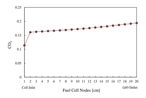
Figure 6.14. CO<sub>2</sub> profile across the fuel cells
