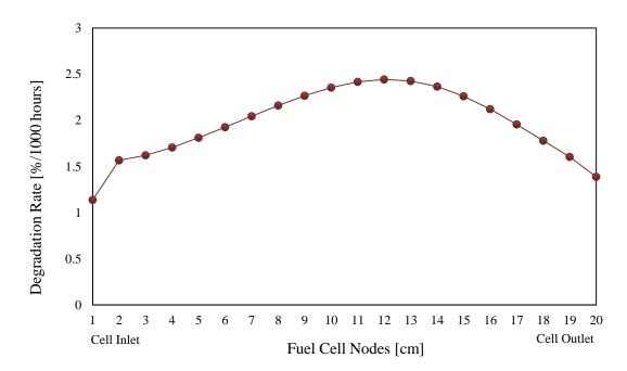
Figure 6.7. Degradation rate profile across the fuel cells
