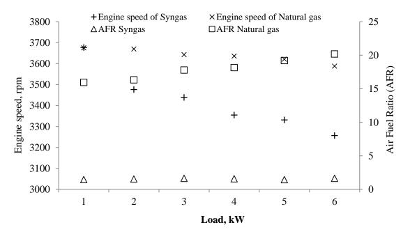
Figure 2.3. The engine speed and AFR with varying load for engine using syngas and natural gas (note that load on natural gas fuel continued to increase until 9 kW)
