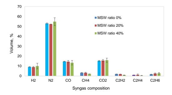
Figure 3.2. Gas composition of syngas generated at various MSW ratio (0, 20, and 40 wt.%) at maximum load (5 kW)
