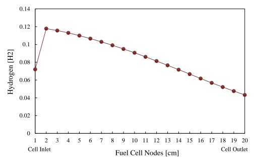
Figure 6.10. H<sub>2</sub> profile across the fuel cells
