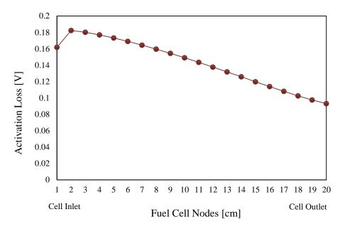
Figure 6.15. Activation loss profile across the fuel cells
