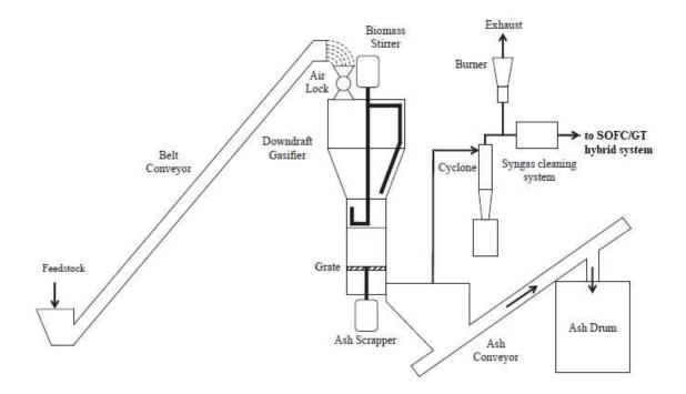
Figure 6.3. Schematic process of gasification plant, consisting of belt conveyor, air lock, biomass stirrer, downdraft reactor, grate, ash scrapper, ash conveyor, ash drum, and cyclone separator.
