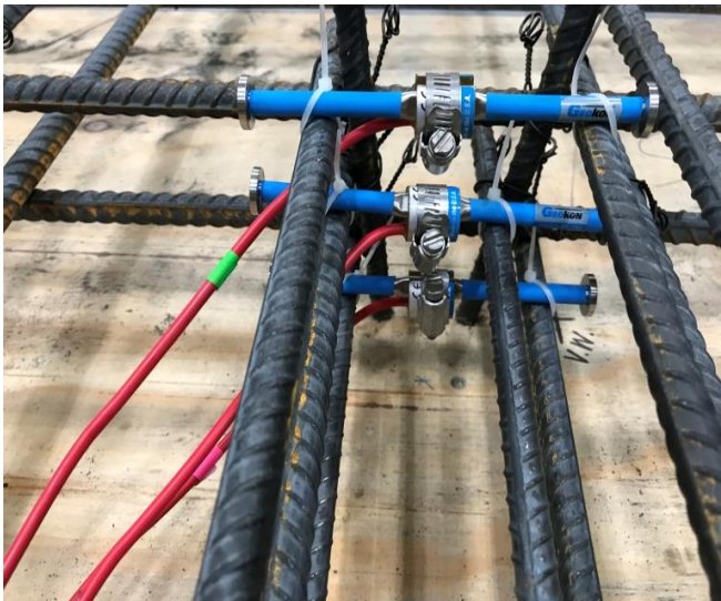
Figure 3.5 - Photographs of VWSG used for data collection: VWSG were placed at 2 in., 4 in. and 6in. depths.
