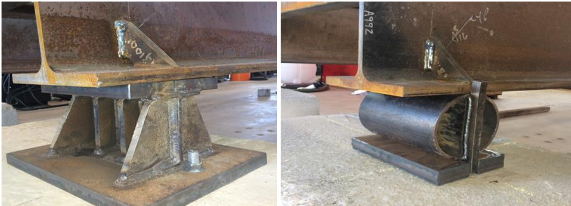
Figure 4.1: Bridge Support Conditions
