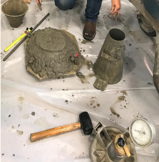
Figure 3.7 - Performing slump test on bridge deck concrete
