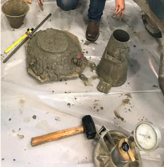
Figure 4.7 - Performing slump test on bridge deck concrete
