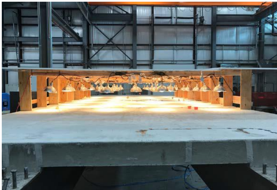
Figure 4.8 - Photograph of Thermal Loading Testing Frame Setup
