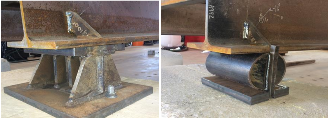
Figure 3.1: Bridge Support Conditions
