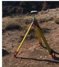
Figure 7: The RTK base station on top of the mesa.
