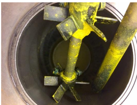
Figure 2.8 An example of the insoluble yellow solid found on the internal components after a successful reaction
