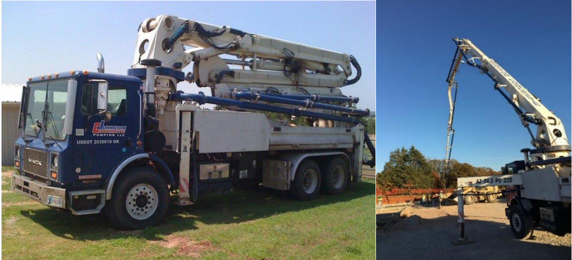
Figure 2-3 – Pumpstar AZ-34.5 / PS-220 Truck Mounted Concrete Pump used in the field-testing.
