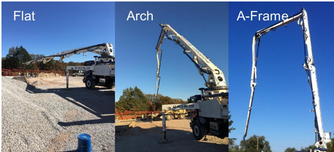
Figure 2-7 – The flat, arch, and A-Frame orientations of the concrete pump.
