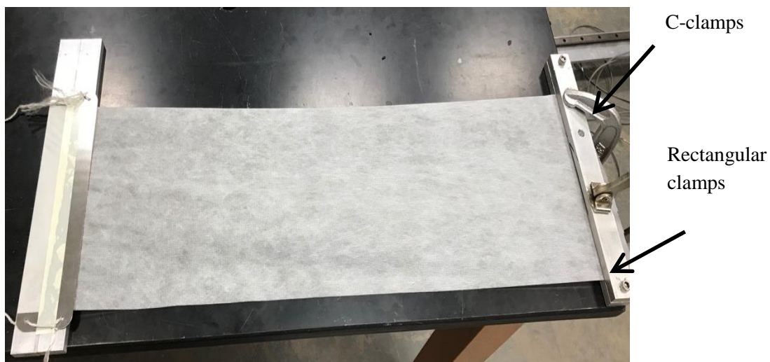
Figure 3.17: Experimental setup of trough test
