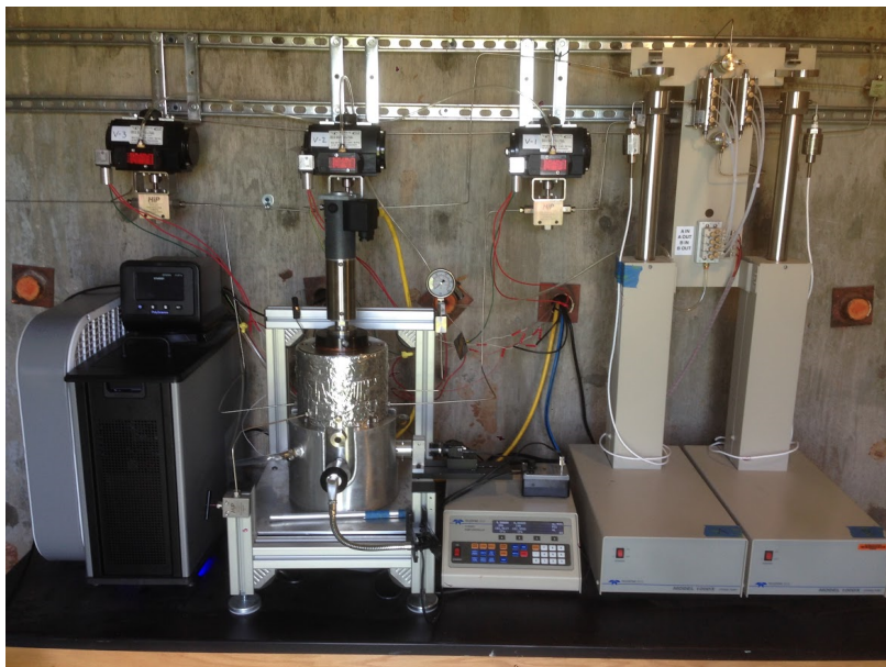
Figure 5.6: Gas evolution experiment located inside the blast cell
