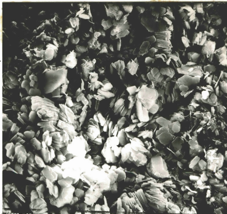
Figure 49. SEM Image of Pore-Filling Kaolinite (CSM-1452, 2000X).
