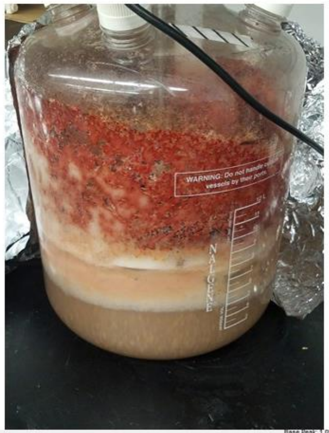
Figure 31: Bioreactor of Spaceloma corylii . A large quantity of medium, 10L, was able to be inoculated and grown in a single container with increased air flow.
