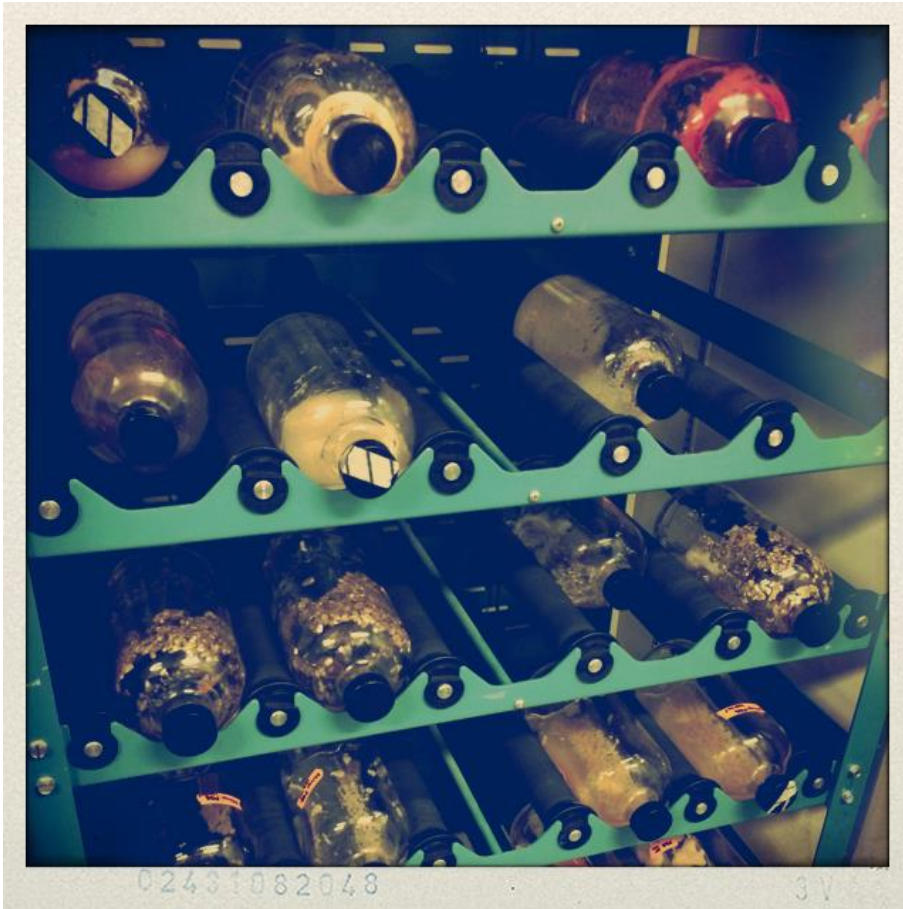
Figure 29. Photo of Roller Bottles. A device that slowly rotates bottles, potentially allowing greater surface adhesion of growing organisms.
