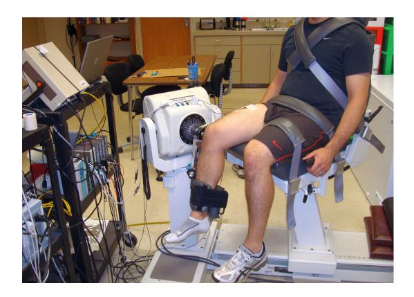
Figure 4. Dynamic constant external resistance assessment set-up.
