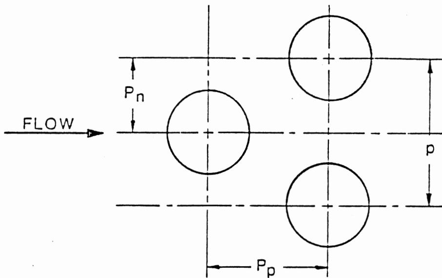
Figure 4. Tube Pitches Parallel and Normal to Flow (4)
