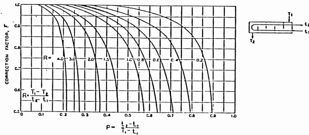
Figure 1. LMTD Correction Factor For an Even Number of Tube Passes (5)
