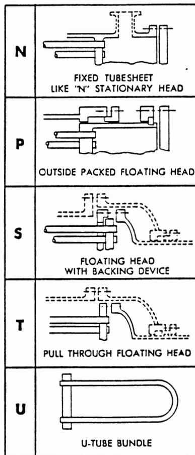
Figure 3. Tube Bundle Construction (5,14)
