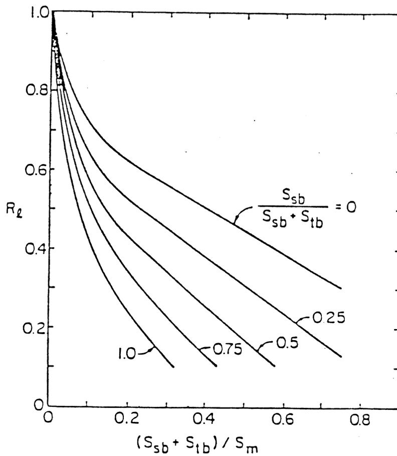
Figure 13. Correction Factor For Baffle Leakage Effect on Pressure Drop (4)
