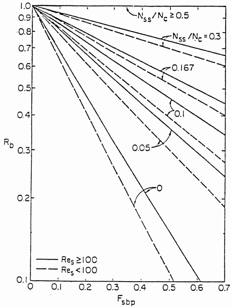
Figure 14. Correction Factor on Pressure Drop for Bypass Flow (4)
