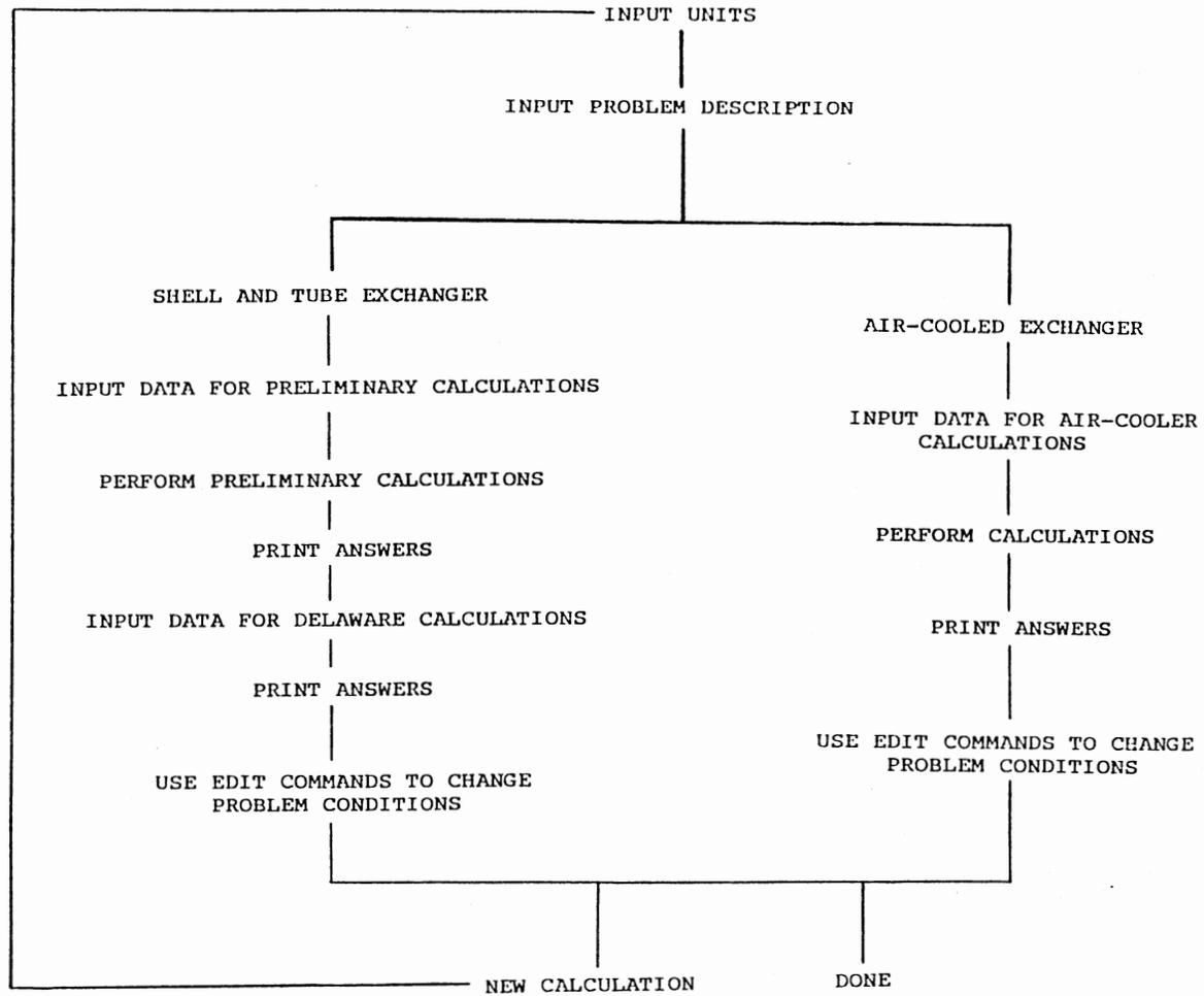
Figure 1. Logic Diagram for HEXSIM
