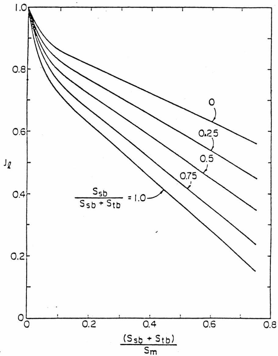
Figure 7. Correction Factor for Baffle Leakage (4)
