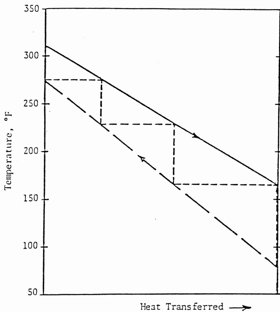
Figure 2. Estimation of Required Number of Shells in Series (4)
