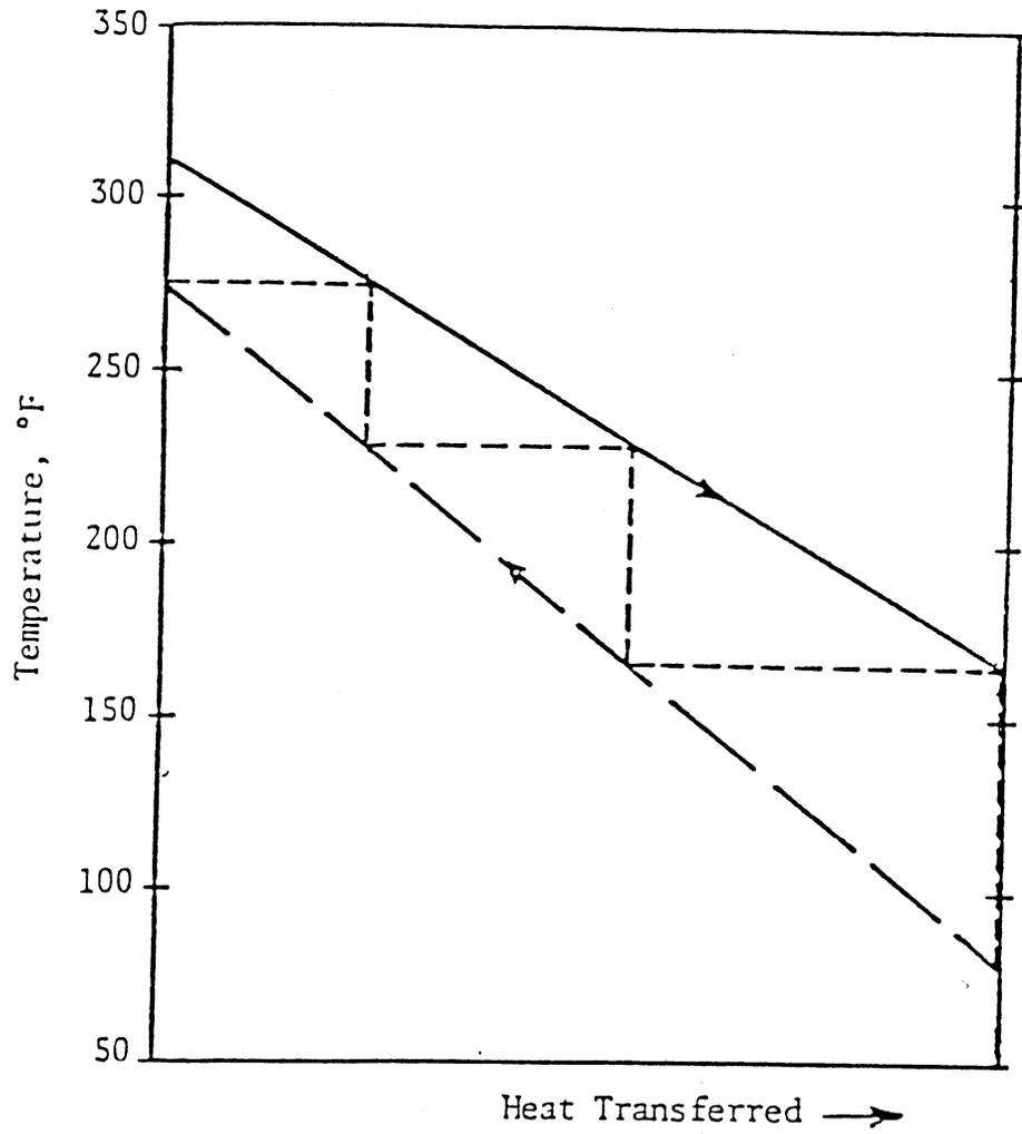
Figure 6. Estimation of Required Number of Shells in Series (5)
