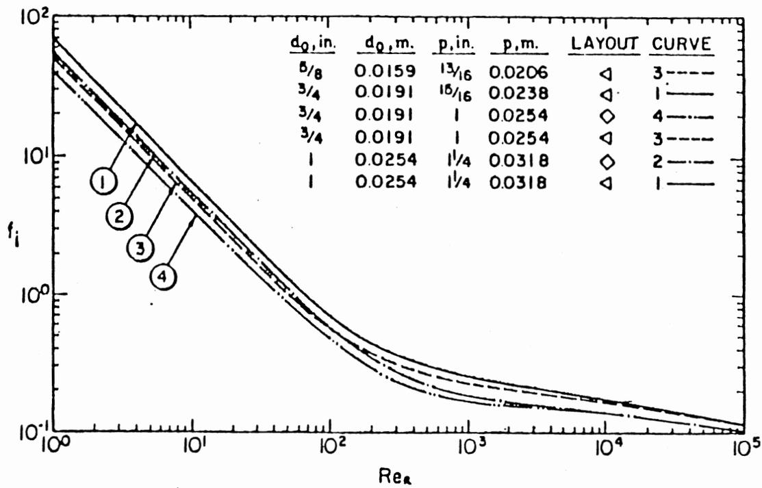
Figure 11. Correction of Friction Factors For Ideal Tube Banks (4)
