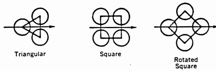
Figure 2. Tube Arrangement (14)
