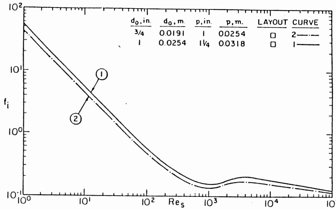
Figure 12. Correction of Friction Factors For Ideal Tube Banks (4)
