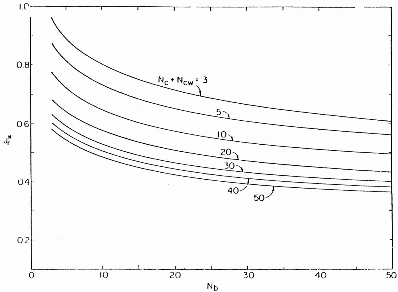
Figure 9. Correction Factor For Adverse Temperature Gradient at Low Reynolds Number (4)
