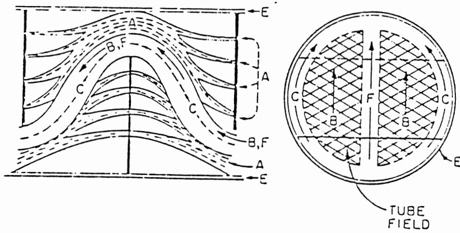
Figure 3. Idealized Diagram of Shell-Side Flow (4)
