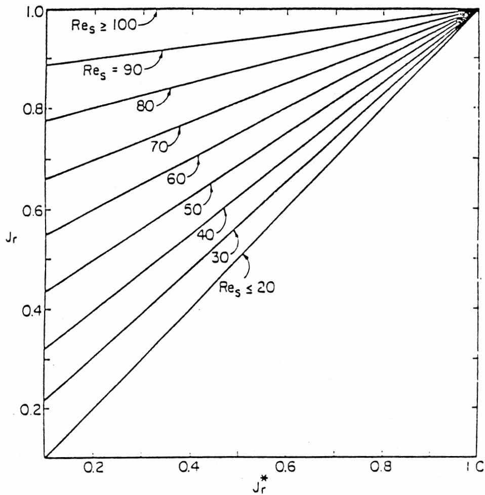
Figure 10. Correction Factor For Adverse Temperature Gradient at Intermediate Reynolds Number (4)
