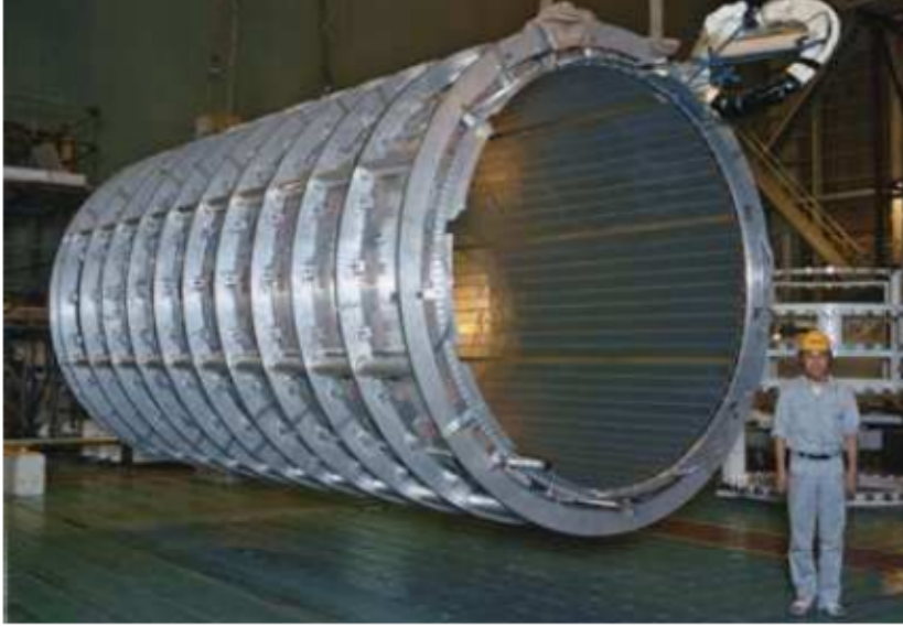
Figure 3.3: The solenoid magnet of the ATLAS detector (43).
