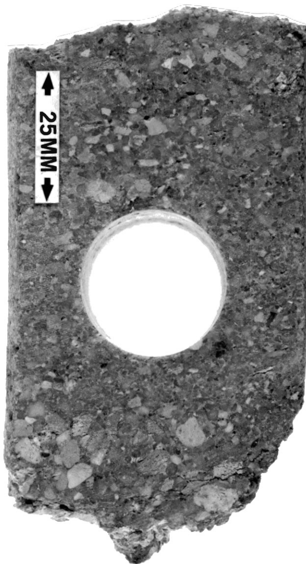
Figure 13. One Fining-Upward Sequence of a Braided Stream Deposit Within the Apache Gregory Core at 17,180 Feet.
