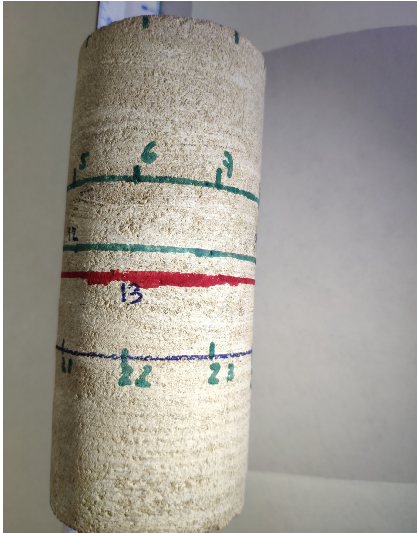
Figure A-1-9. Portions of the rock sample with a difference in the porosity distribution. Red line represents the middle of the sample.
