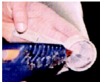
Figure 6E. Seal two layers of screening together.
