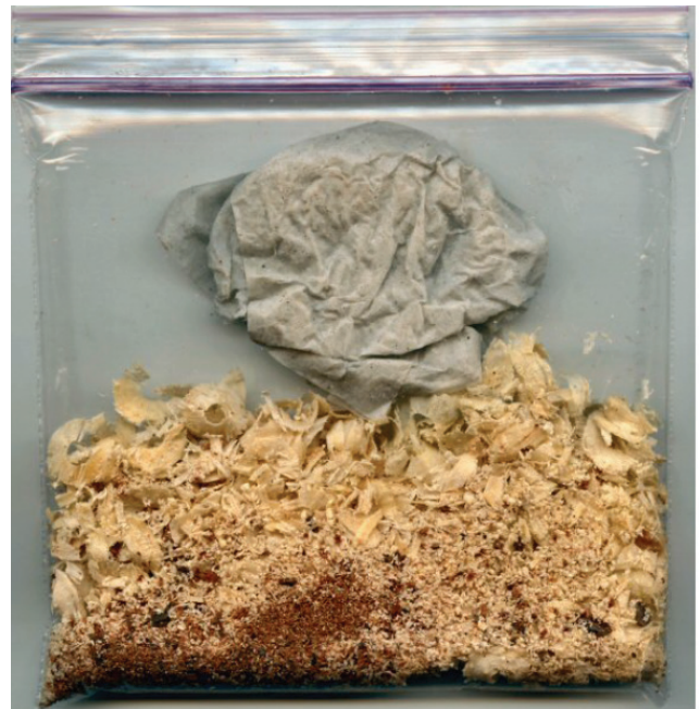
Figure 6. Store wood chips or shavings in a sealed plastic bag with a damp paper towel in the refrigerator until shipment.
