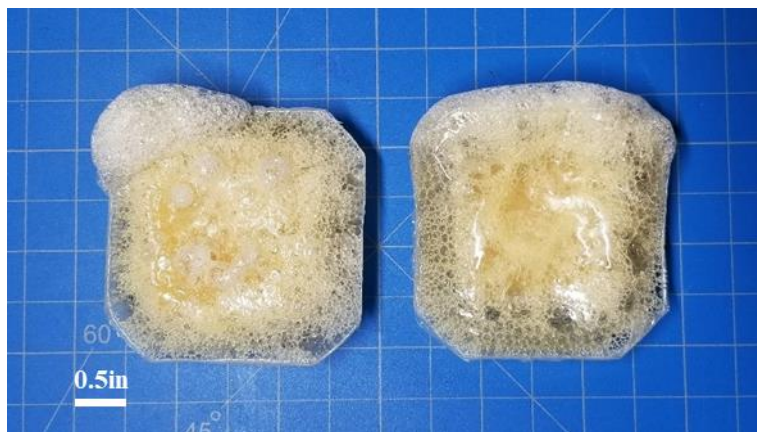
Figure A1.5: Cured SMP cast around a sugar scaffold in the shape of a weigh boat
