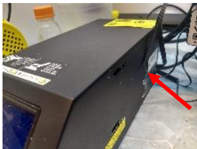
Figure A2.1: Location of the SD card slot on the printer control box.
