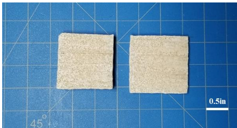
Figure A1.6: Same SMP blocks from Fig. A1.5 with all excess polymer trimmed away.
