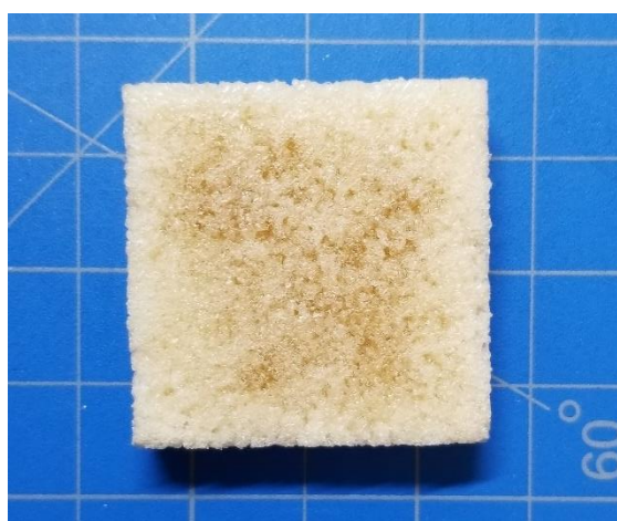
Figure A1.7: Same SMP block from Fig. A1.6 showing partial sugar dissolution. Note that the dark shading in the center indicates the presence of remaining sugar.
