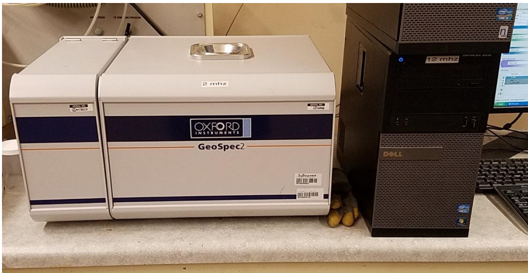
Figure 2.7: The Oxford GeoSpec2 NMR spectrometer used in present study operates at 2 MHz and has a minimum echo spacing of 57 \mu s.
