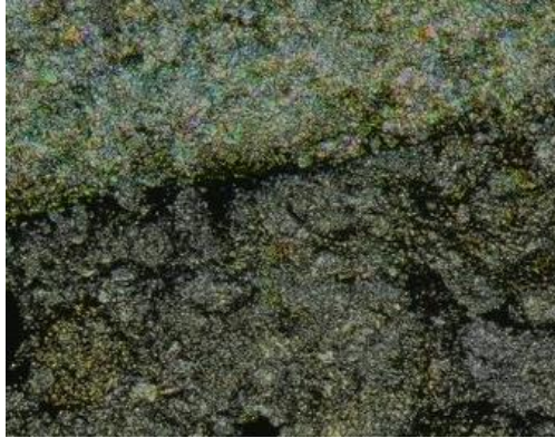
Figure B9 – Microscope images at different points of the interface between Neat class H cement (bottom layer) and shale (top layer)
