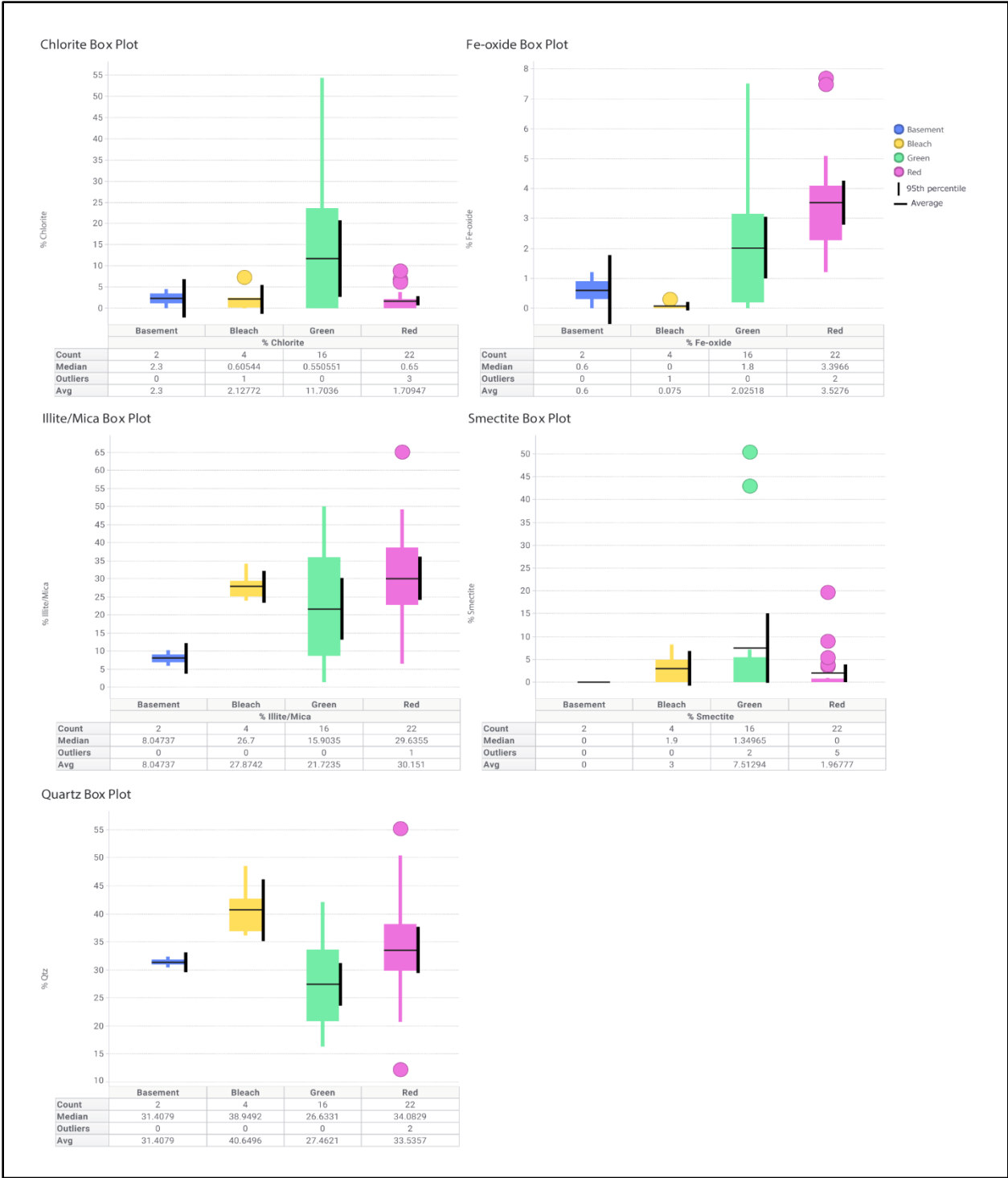
Fig. 11: Box plots comparing the mineralogical abundance of five key minerals in the RGB + basement samples.
