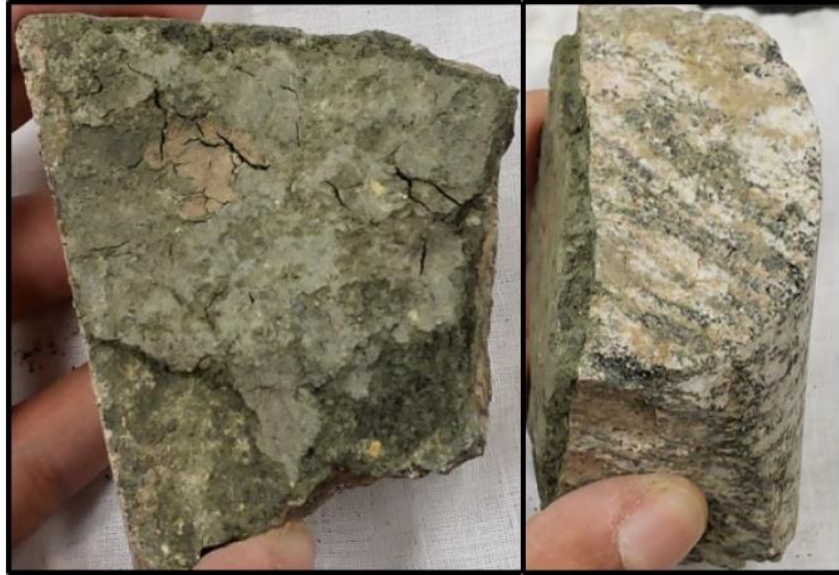
Fig. 12: Images of Massey core #1 sample MC-01-1078, containing green clay hosted within a gneissic basement rock fracture.
