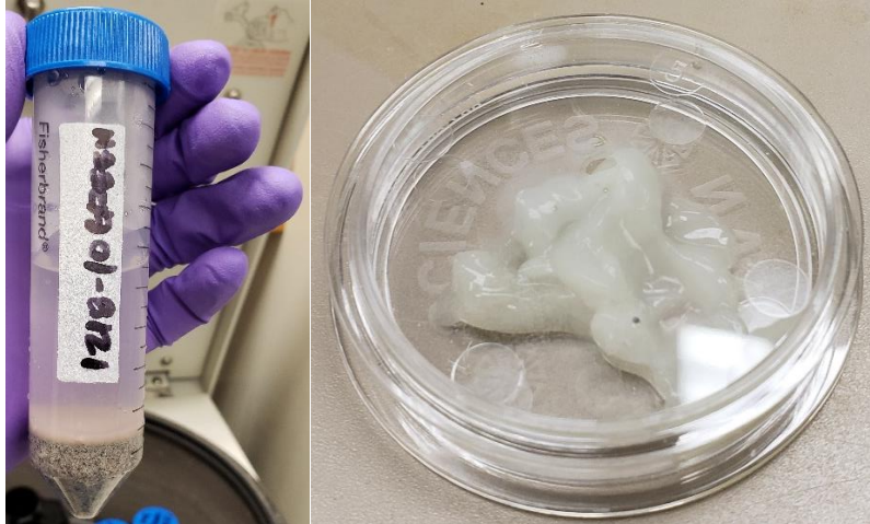
Fig. A2: Swelling clay “goo” from CBD treatment when preparing samples for LPSA. Goo is identified as smectite in Fig. A3 and was fixed by cooling the samples in an ice bath overnight.
