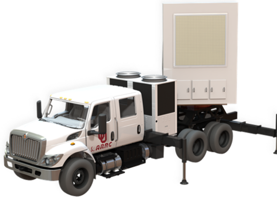
Figure 4.1: Conceptual drawing of the Horus radar [4].
