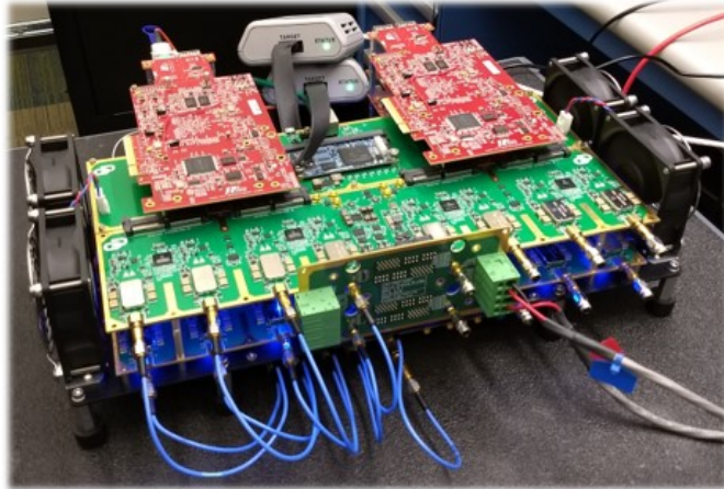
Figure 4.2: Test bench setup for the data collected from this experiment. The signal is passed through four channels of one of these “Octoblade” receivers.
