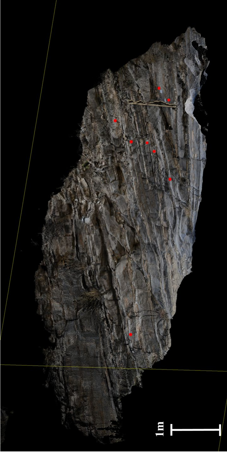
Figure 36: True color point cloud image from Split-FX. Red infilled circles denote XRF/Schmidt Hammer measurement positions 1-7. Unconformity identified above measurement position 2.
