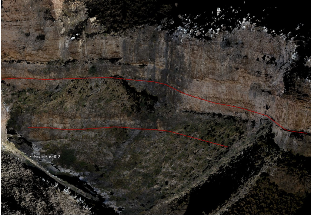
Figure 15: Point cloud data displayed in true color. Also shown is scan position 002 and formation boundaries of the Bone Spring/Cutoff formations (bottom line) and Brushy Canyon/Cutoff formations (Top line)
