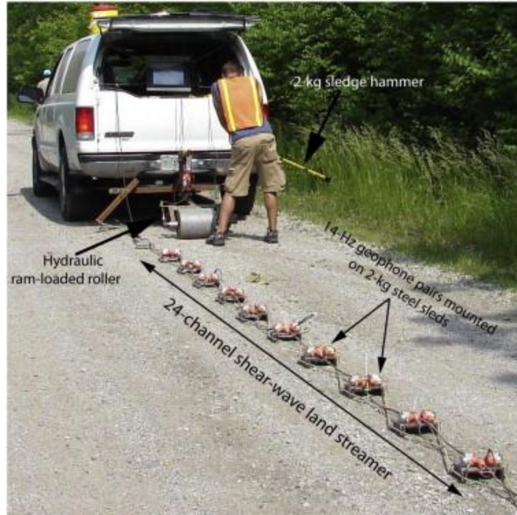
Figure 4.1: Field photograph illustrating the components and layout of the SH-wave land streamer seismic acquisition method (Ismail et al., 2014).
