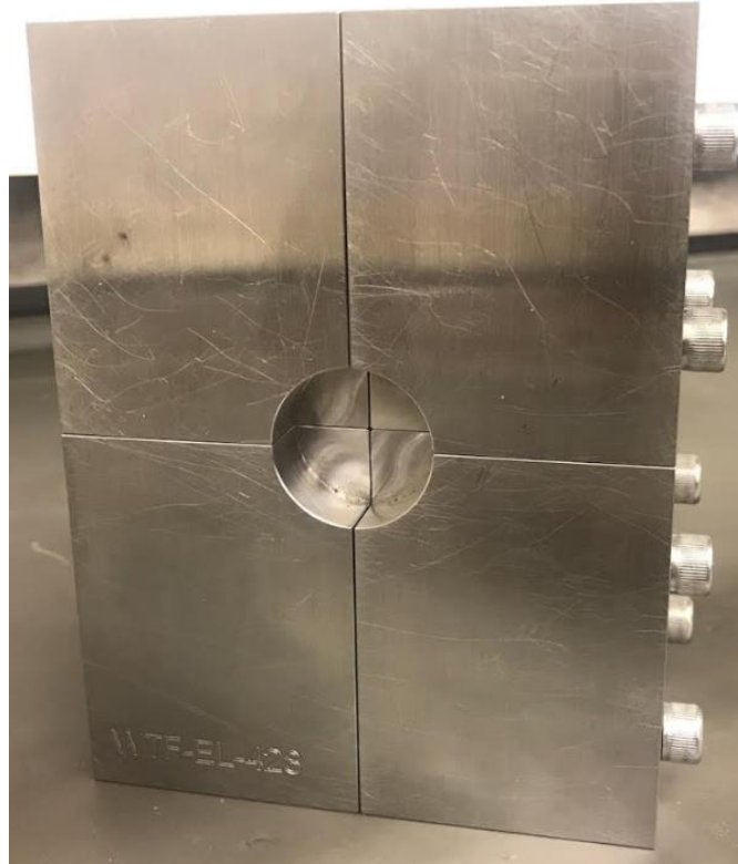
Fig 2.9 Combined Loading Compression (CLC) Test Fixture (ASTM D6641)
