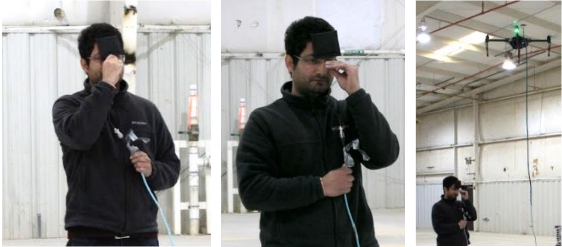
Figure 3.3 A standing human subject with UWB antenna patch attached to his forehead with the transmitter to the UAV in the indoor warehouse environment.
