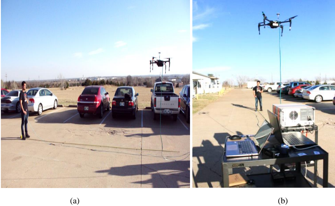
Figure 2.13 Outdoor setup with human subject and in the LOS (a) side view of the setup with patch on his wrist (b) front view with patch location on his wrist.
