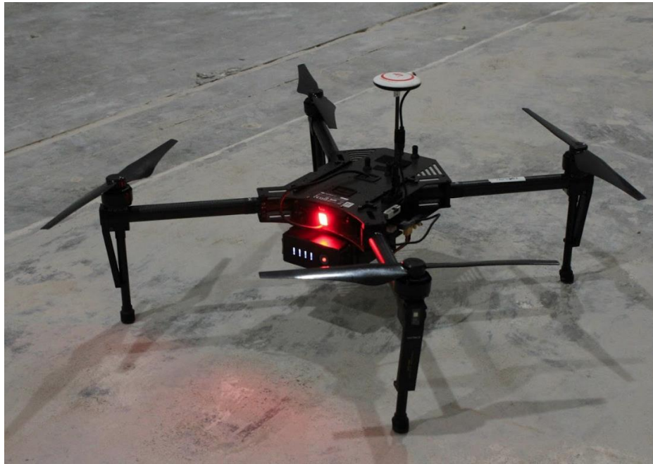
Figure 2.8 An IRIS+ quadcopter used for placing the transmitter.
