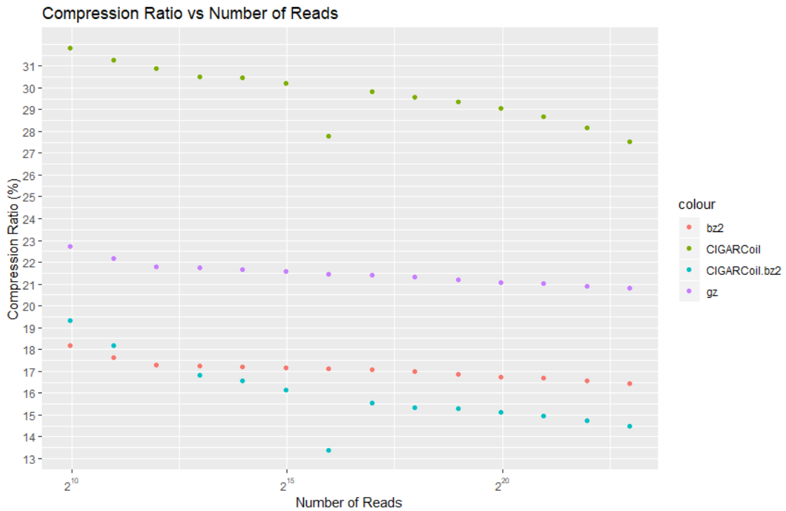
Figure 4.3: Compression Ratio vs Number of Reads With Clustering Performed on Reads from Beginning of the SRX001540 Dataset
