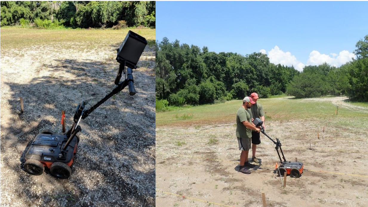
Figure 5.5: GSSI UtilityScan GPR unit with Android tablet display (left), grid set up for GPR survey in the west bait field (right)
