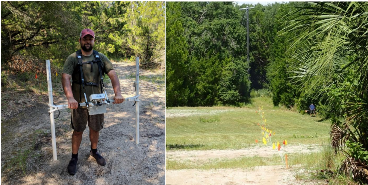
Figure 5.3: Bartington 601 Magnetic gradiometer with dual sensor array (left), pin-flags set-up for data collection (right)
