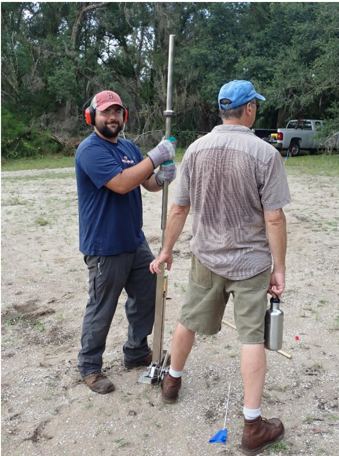
Figure 5.6: ESP core device in use. A manual slide hammer drives the metal probe with copolyester tube into the soil, taking a slightly compacted version of real stratigraphy.
