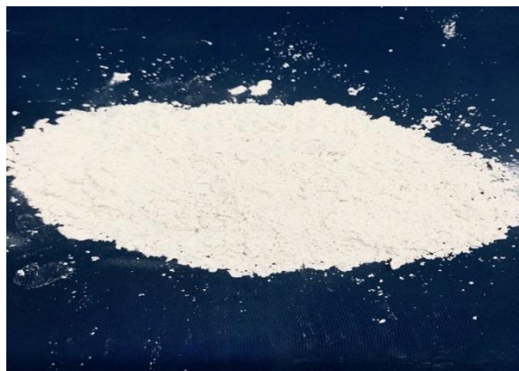
Figure 4.7. BaTiO 3 powders; particles with nominal diameter of 400 nm before packing
