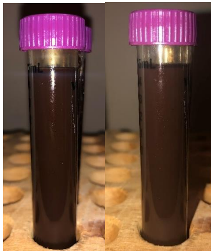
Fig. 21—30% water-cut (left) showing separation after 30 minutes (right)
