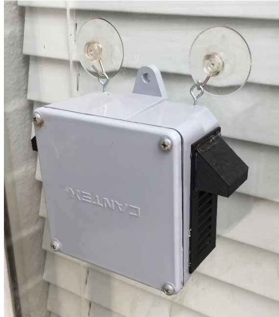
Figure 2.15: Photo of outside air temperature sensor case
