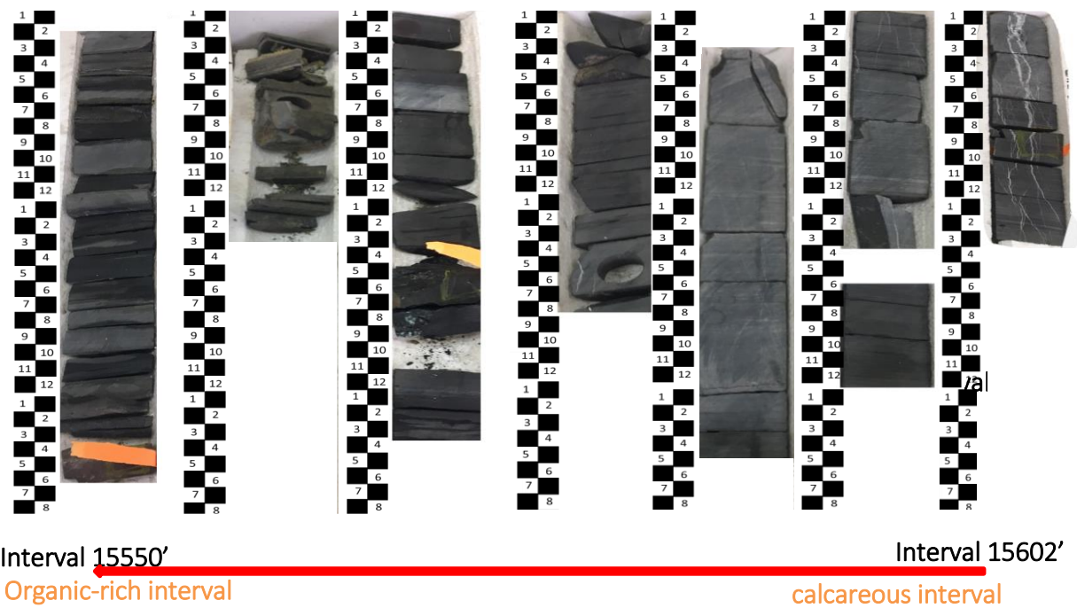
Figure 15. LLIE core interval displaying gradually lithological changes (calcareous to organic-rich mudstone). There is also a presence of erosion surfaces and lag deposits.
