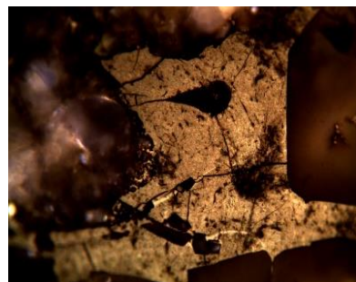
Grainy bitumen, 1,01%Ro
