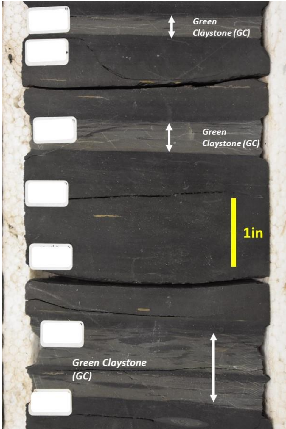
Figure 46 Example of Green Claystone (GC) interbedded with Argillaceous Shale (AS). They show mottled texture like in the lower bed implying bioturbation activity during or after deposition. These GC beds tend to thin upward in the section. They are located in the lowermost part of the core.
