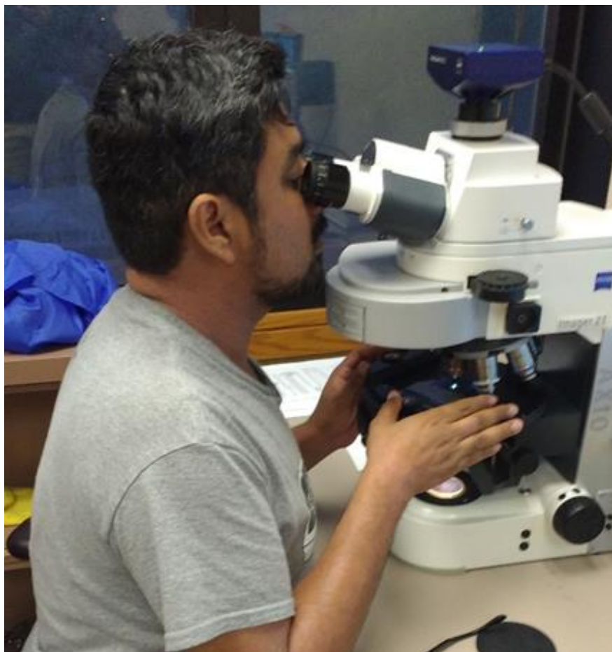
Figure 66 Picture of graduate student (Antonio Cervantes) looking in the Carl Zeiss AX10 Imager Z1 petrographic microscope. It has the capability of using 1) transmitted plain-polarized light (PPL), 2) transmitted cross-polarized light (XPL), and 3) reflected light (RL). This instrument is property of ConocoPhillips School of Geology and Geophysics (CPSGG) at The University of Oklahoma (OU).
